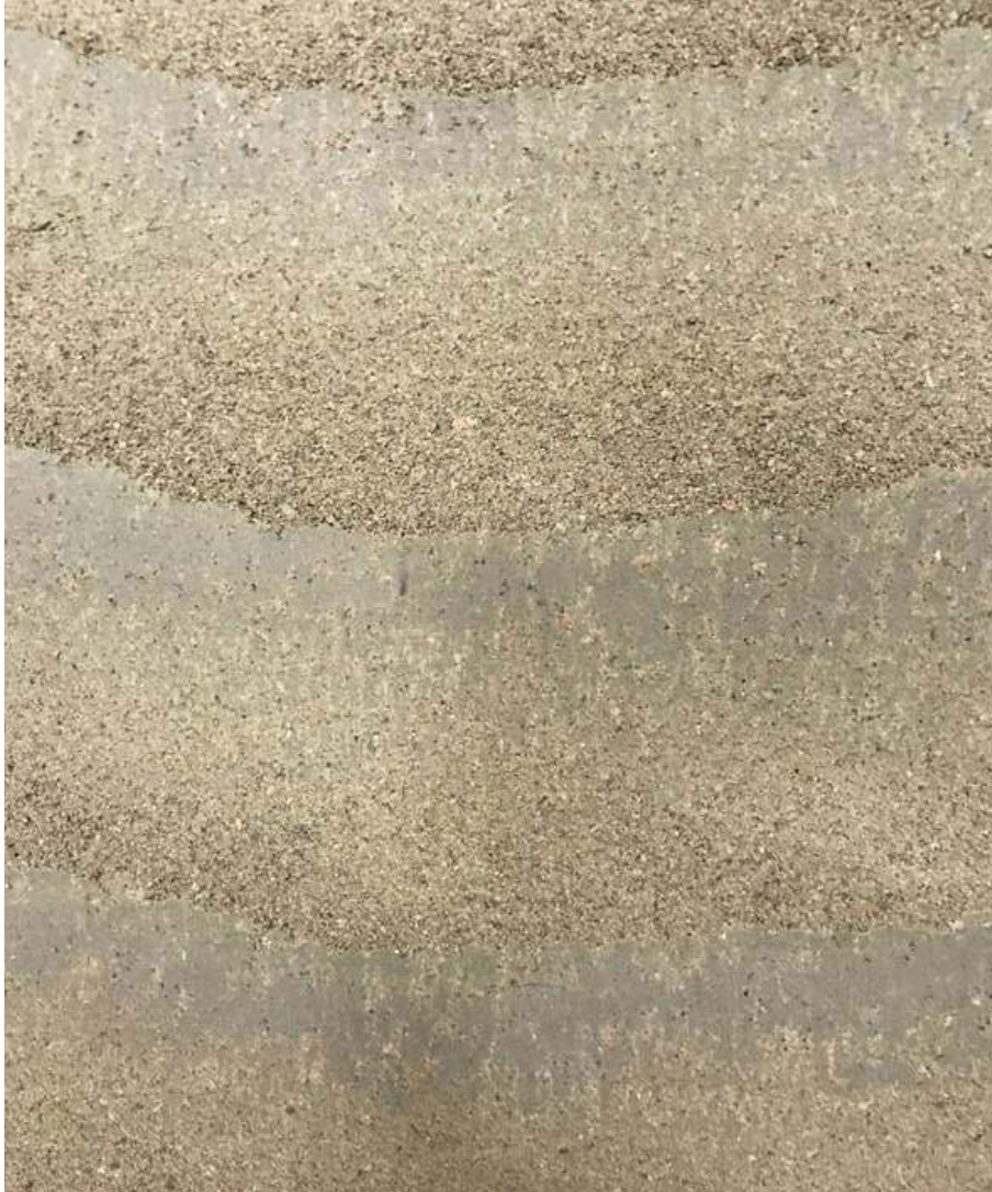
Image 1. Rammed earth sample realized by the EarthLAB and the Author, using clay from Göteborg (Picture: Author, 2020)
