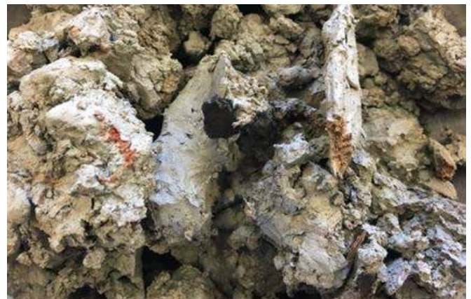
Image 4. C1, Clay from central station (Picture from ZRS, Personal communication, 2020)
