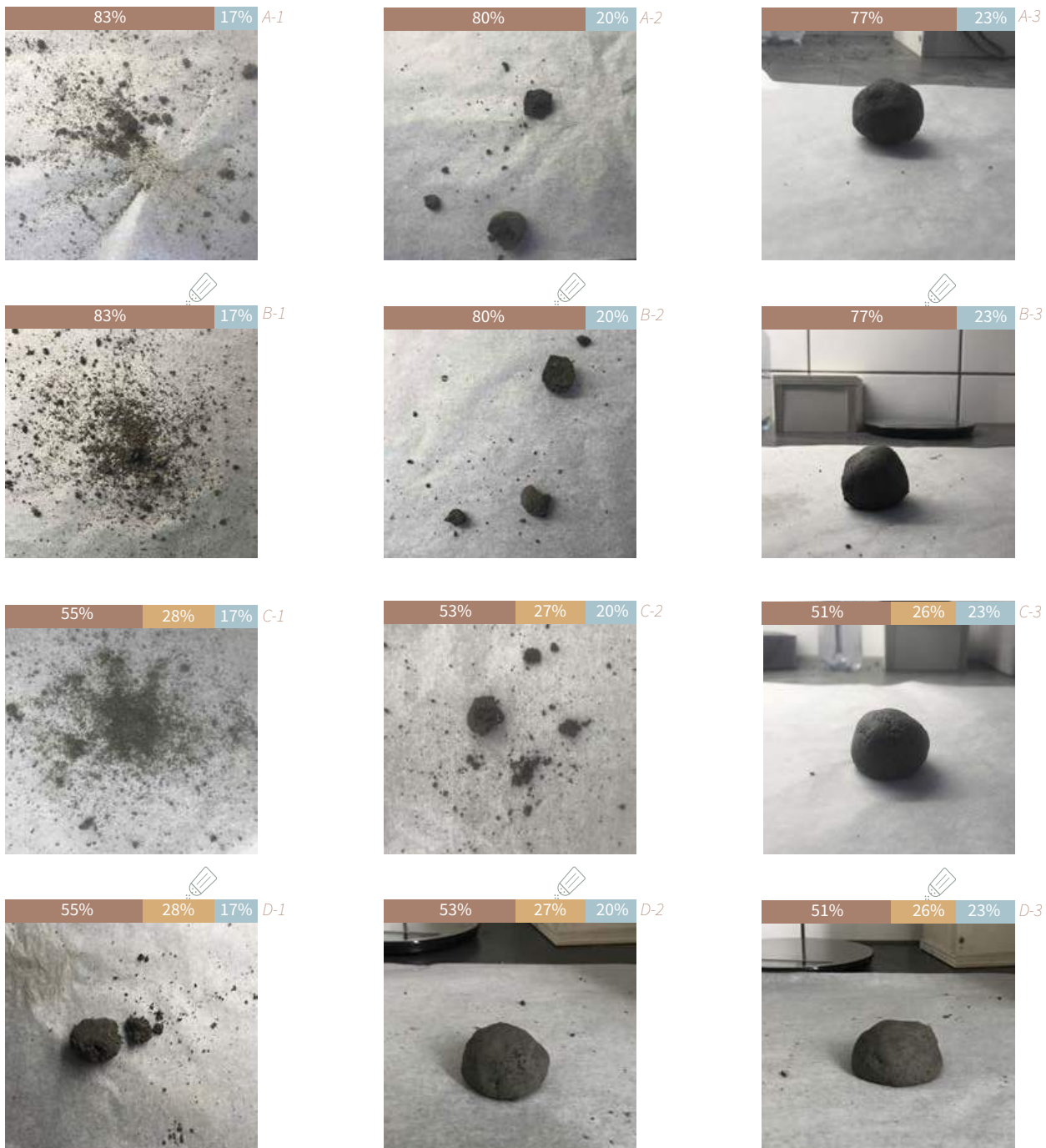
Image 9. Drop test with different mixtures ((Pictures and tests by the author))
