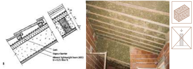
Image 36. Left Roof infill details (Minke, G. 2009)
