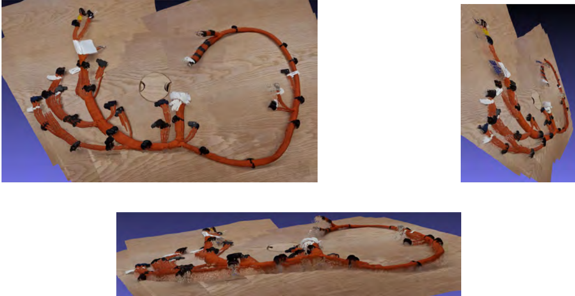
Figure A.5: 3D segmented views of the orange wire harness for Pi3
