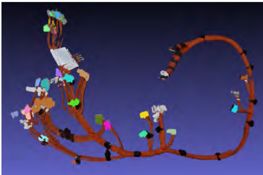
(a) Classifying terminal housings with a Map Anything reconstruction.
