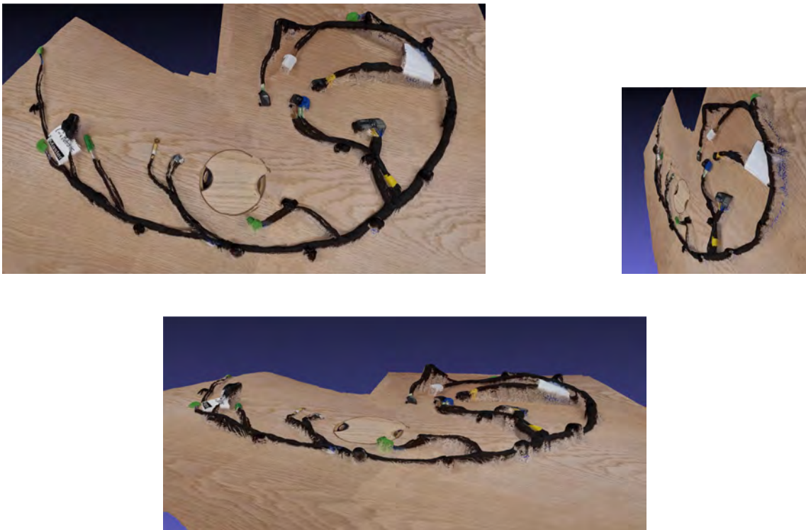
Figure A.6: 3D segmented views of the black wire harness for Pi3
