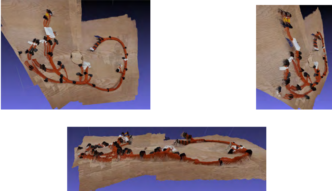
Figure A.3: 3D segmented views of the orange wire harness for Map Anything
