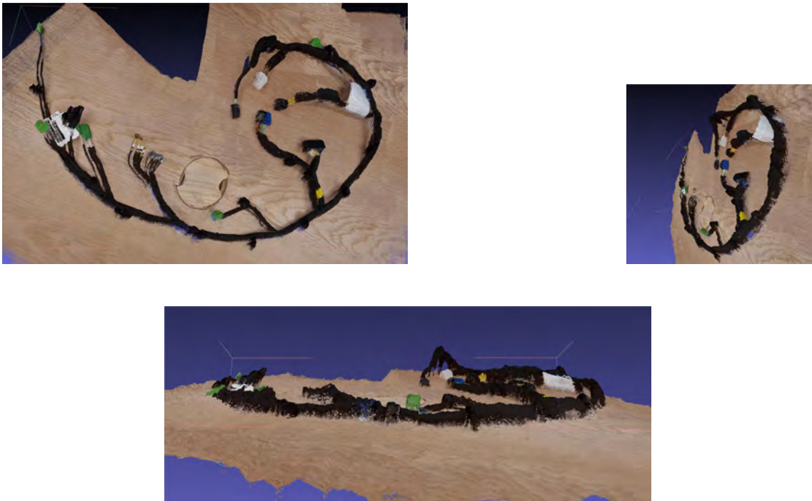
Figure A.4: 3D segmented views of the black wire harness for Map Anything
