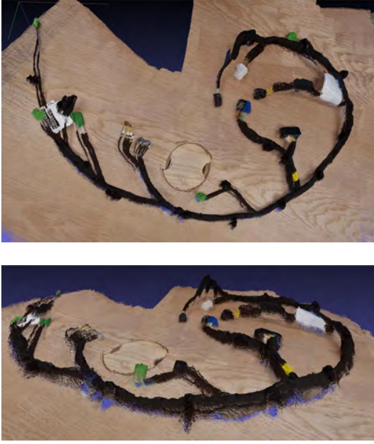
Figure 4.3: 3D reconstruction from Map Anything of the black wire harness
