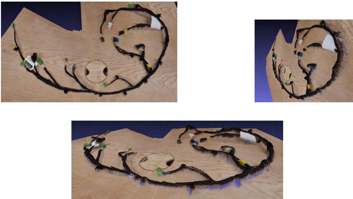
Figure A.2: 3D segmented views of the black wire harness for DA3
