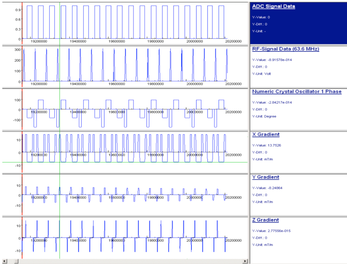
Figure 3.2: Self programmed balanced SSFP sequence diagram from the IDEA POET simulator.
