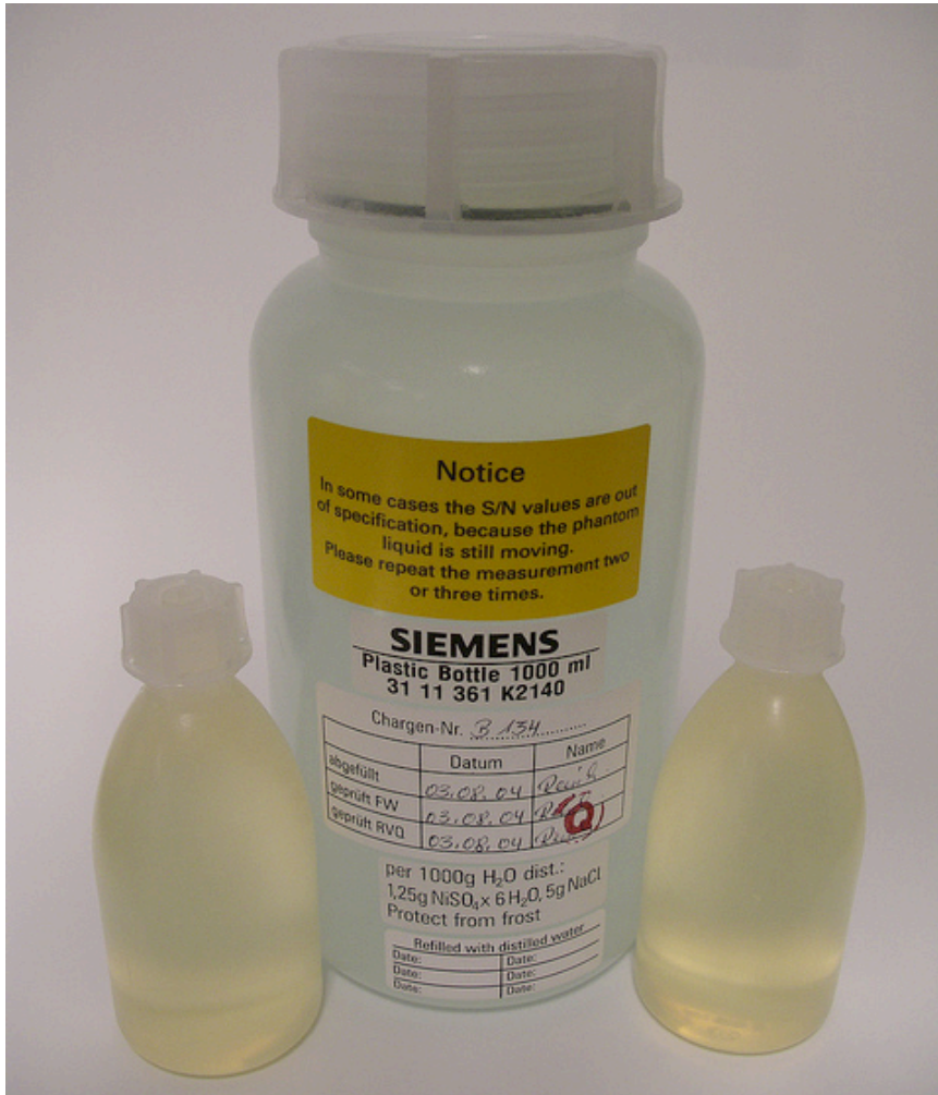
Figure 4.2: Measuring object for the optimization were a Siemens standard water phantom and two smaller bottles filled with sunflower oil.
