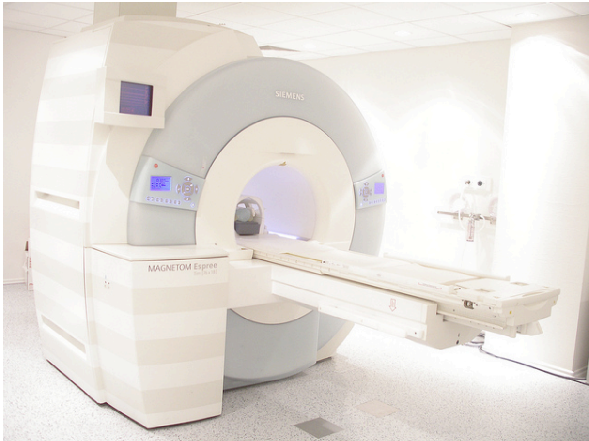
Figure 4.1: The Siemens MAGNETOM Espree 1.5 Tesla clinical MR-scanner used for the optimization of the sequence.
