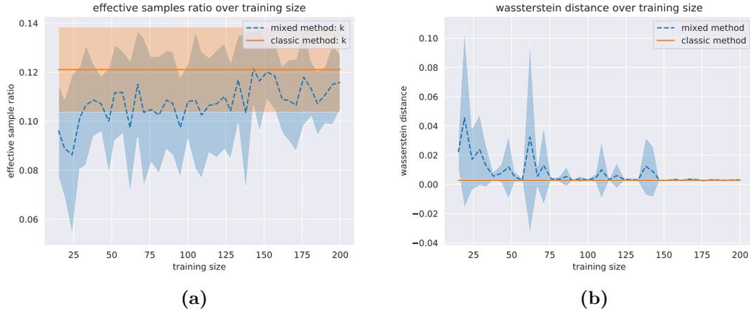
**Figure 6.5:** The performance metrics over training data sizes. Figure 6.5a illustrates the *ratio* of effective samples per iteration against the training data size for the MMH. Figure 6.5b likewise illustrates the WD against the training data size for the MMH. The shaded regions are the standard deviations of the metrics. In both figures, the benchmark CMH algorithm metrics are also plotted.
