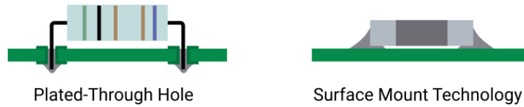
Figure 2.1: Electrical components placed with PTH and SMT.
