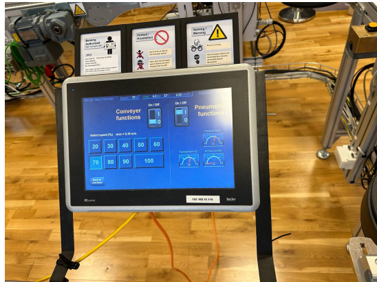
(a) Photograph of the HMI touchscreen at the SII-Lab.
