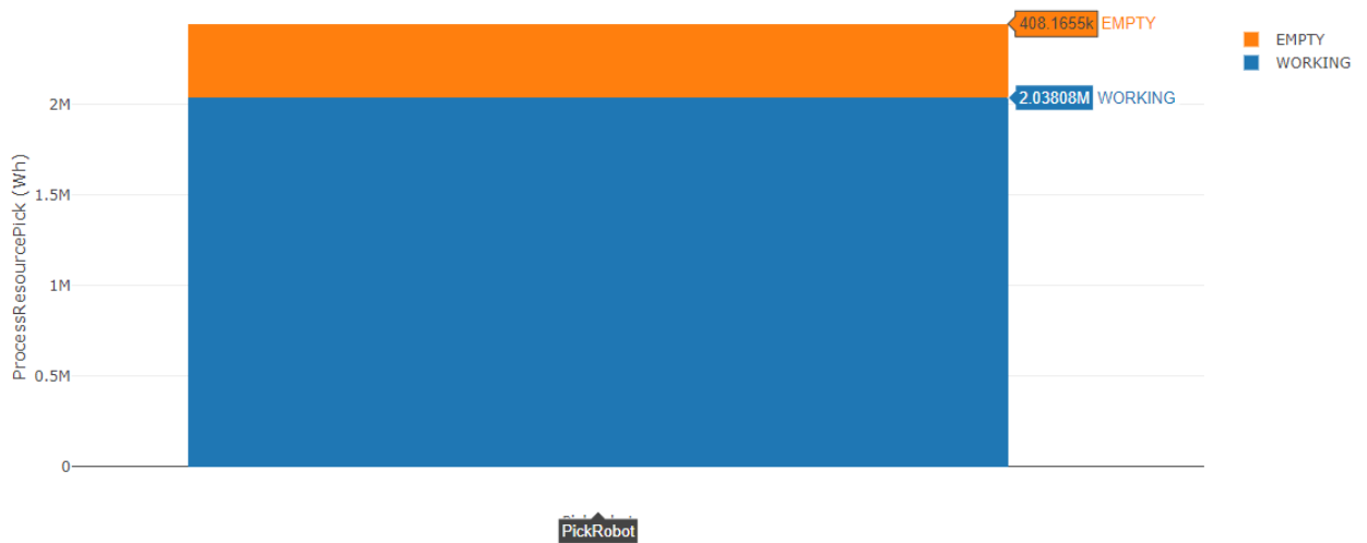
Figure C.8: Energy consumption of pick robot after improvements based on one solution from the Pareto front.
