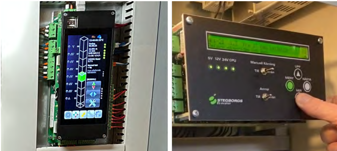
Figure 3.4: Left - Microprocessor controller Thor E2 by Hiselektronik (photograph from lift fair). Right - Microprocessor controller by Stegborgs (photograph from observation).
