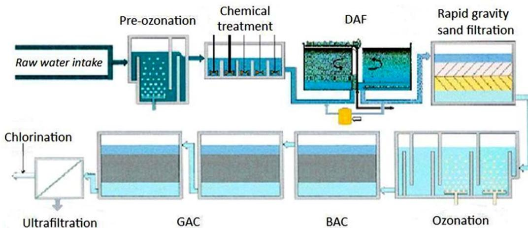
Figure 3 The treatment processes at NGWRP (With permission from WINGOC 2011).
