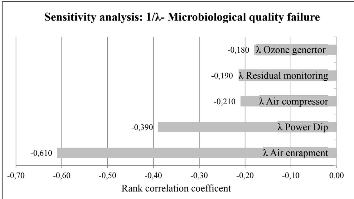
Figure 17 Sensitivity analysis for the uptime of microbiological failure in the fault tree.
