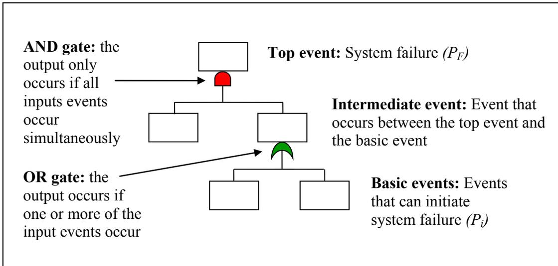
Figure 10 Description of symbols used in fault trees.
