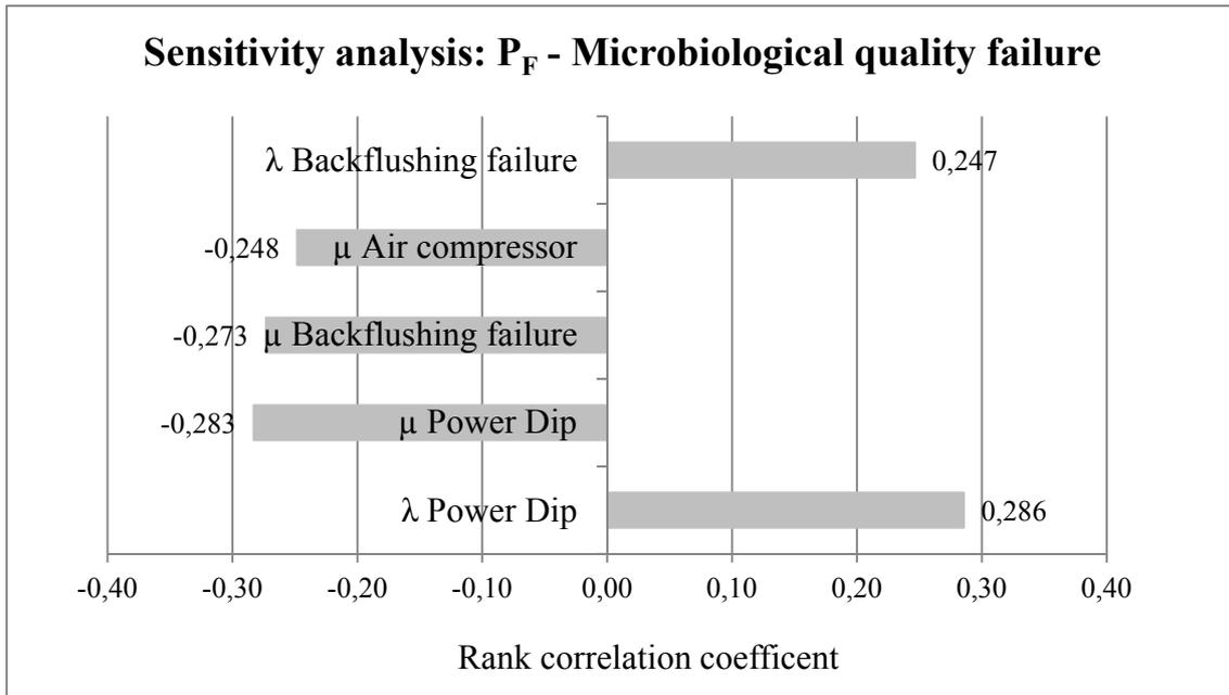
Figure 15 Sensitivity analysis for the probability of microbiological failure in the fault tree.
