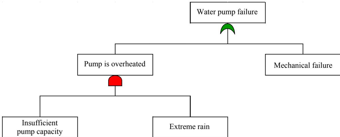
Figure 11 Example of a FTA when there is a water pump failure.
