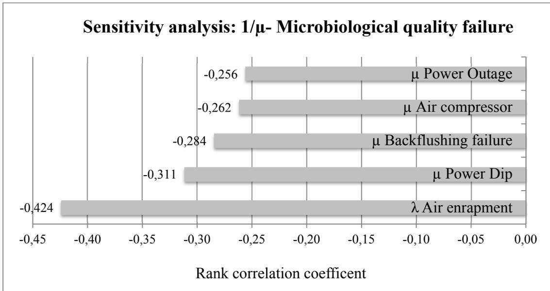
Figure 16 Sensitivity analysis for the downtime of microbiological failure in the fault tree.
