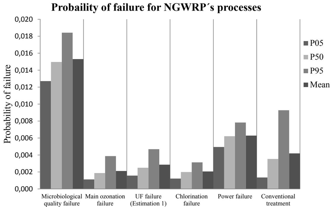
Figure 14 Probability of failure, from the FTA, of the different processes and power failure (presented with 5%, 50%, 95%-percentile values and mean value).
