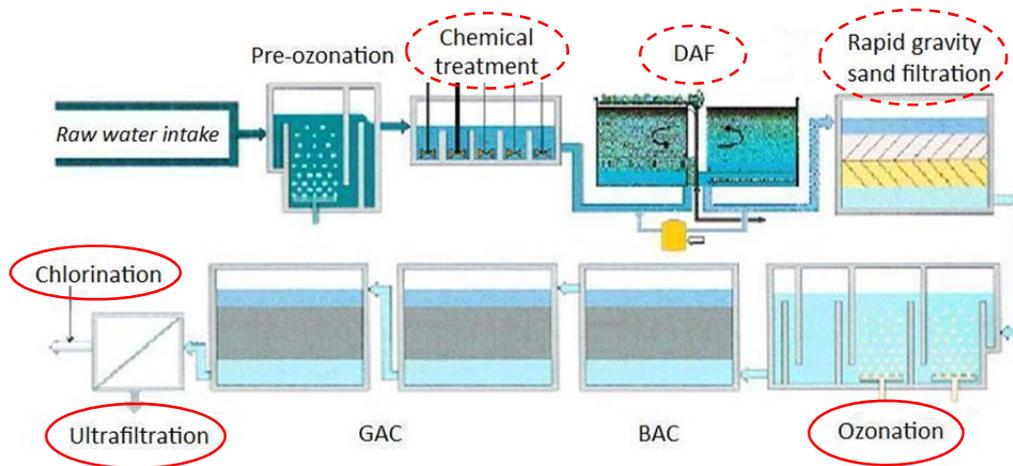
Figure 13 In this Master's Thesis, fault trees were constructed for the process marked with red circles. For those marked with crosshatched red circles fault trees were constructed in an earlier risk assessment.
