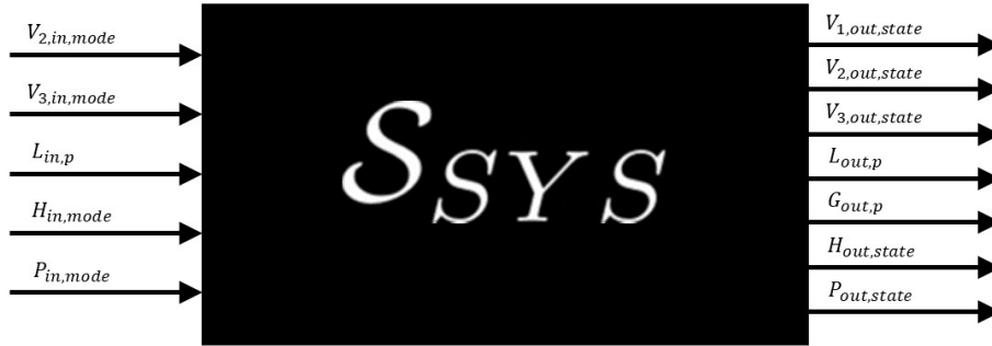
Figure 4.5: Schematic diagram of the black-box model for \mathcal{S}_{SYS} .
