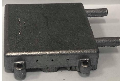
(b) Printed prototype of final concept 3
