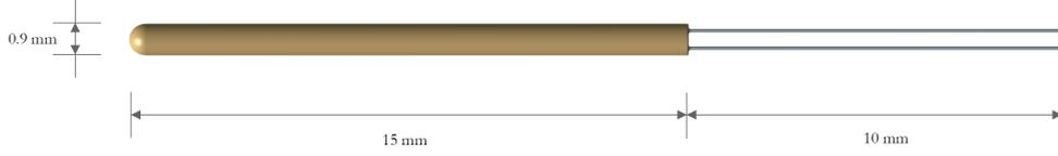
Figure 4.7: Dimensions of the selected Pt100 sensor in 3D
