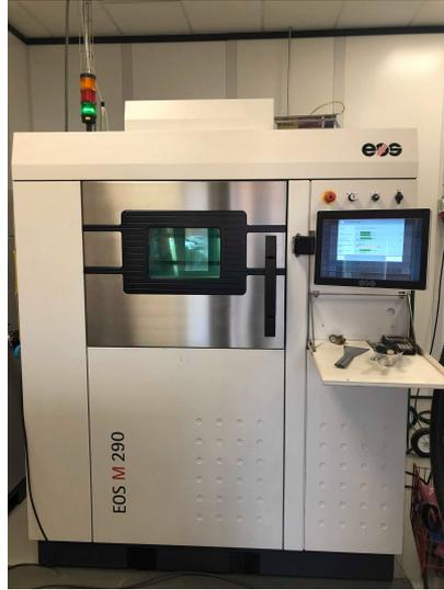
Figure 4.16: EOS M290 machine which was used for printing of the prototypes
