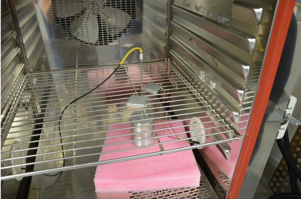
Figure 4.37: The set-up of final concept 1 and 3 in the cooling machine for the functional testing
