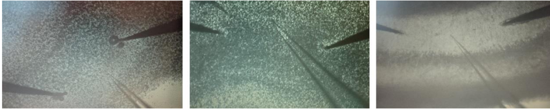
Figure 21. Example pictures of electrode placement in cultured slices (left and middle) and an acute slice to the right. The thick black points are the stimulation electrodes and the transparent one is the recording glass pipette containing the silver electrode submerged in a solution of 1M sodium chloride. In the acute slice to the right, the cinnamon roll-like banded structure of the hippocampus is clearly visible. This makes placing the electrodes where they stimulate the Schaffer collateral axons from CA3 to CA1 in the hippocampus easy. The bands of the cultured slices were less obvious. This degradation was present to various degrees in many of the cultured slices, with the more extreme cases being uniformly grey, making electrode placement much more difficult.
