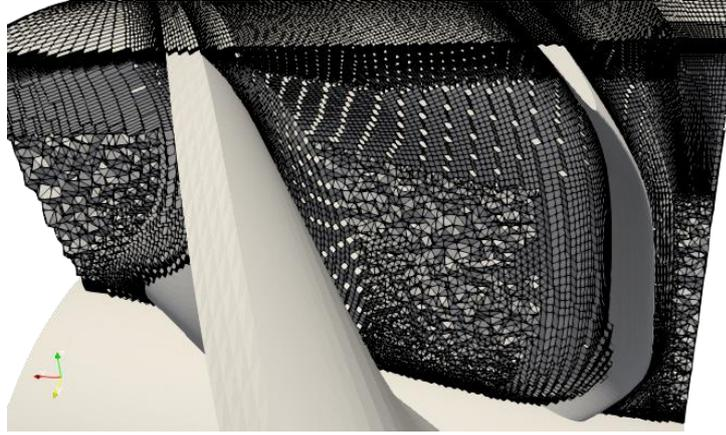
Figure 8. Refined tip mesh to the right and fine mesh to the left at rotor.
