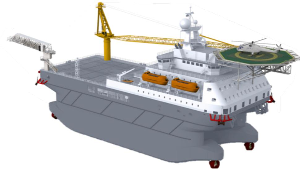
**Figure 2.8:** Compact Semi-Submersible developed by VARD. Adapted from VARD Marine (2018).
