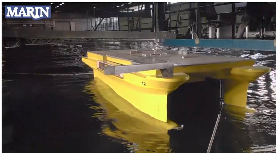
**Figure 2.7:** Windkeeper 5m model at MARIN test basin (MARIN, 2018).
