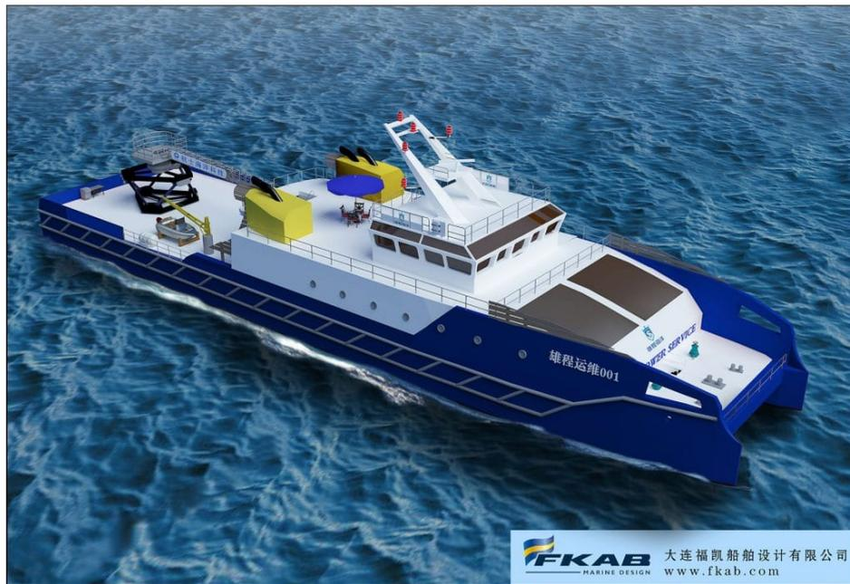
**Figure 2.6:** FKAB 50m offshore wind farm service vessel (FKAB, 2018).
