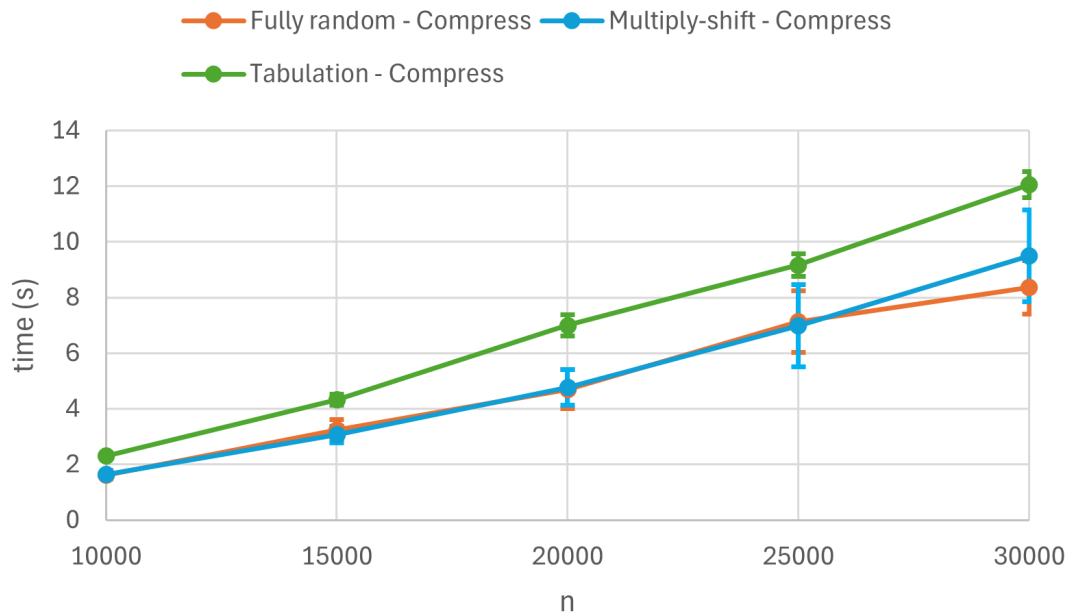
Figure 6.9: Benchmark of the different hash functions with varying values of n on compressed_product_par .
