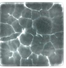
Fig. 33, Cast transparent and white soap, 7 minutes between pouring
