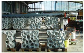
Fig. 27, "Cocoon Club", panellised concrete wall, prefabrication process, design by 3deluxe, development of concrete elements by Villa Rocca
