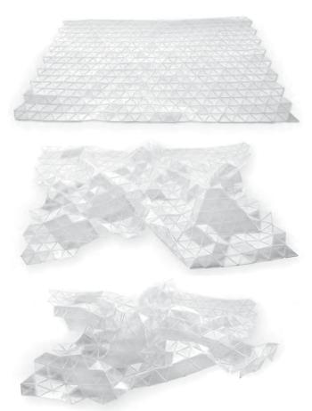
Fig. 114, crumpled surface generation through from flat sheet. Model: Laser cut polyester triangles on adhesive film
