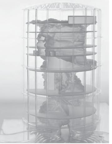
Fig. 119, final design iteration combining the surface and strait edge elements. Model: 3D print in polyamide 2200 and transparent acrylic
