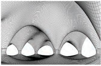
Fig. 46, Kangaroo springs + unary force + anchor points, catenary model generated through Kangaroo (Grasshopper plug-in, Rhino)
