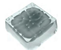
Fig. 40, Cast gel and white soap, 7 minutes between pouring
