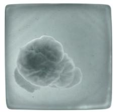
Fig. 35, Cast transparent and white soap, 10 minutes between pouring
