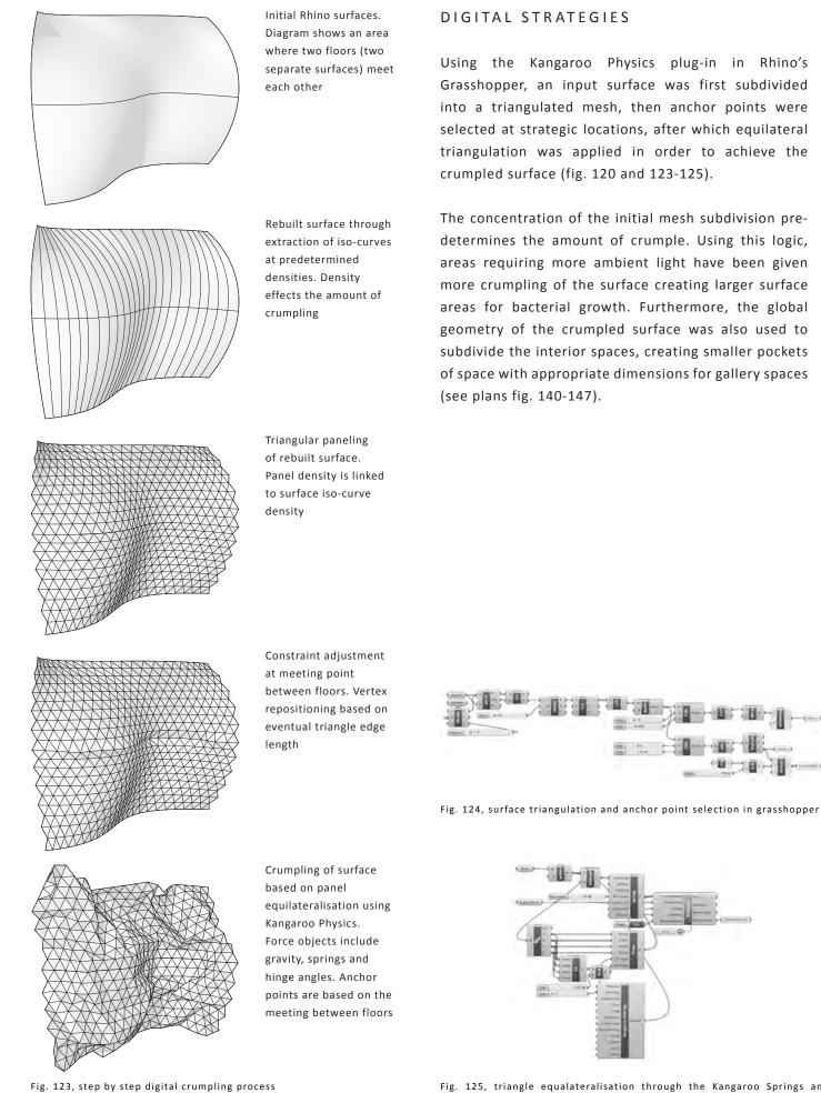
Fig. 125, triangle equalateralisation through the Kangaroo Springs and Hinge forces
