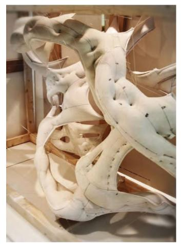
Fig. 10, "Grompies", liquid plaster set in stitched lycra mould, structural design investigation, Brendon Carlin
