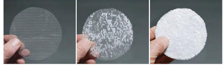
Fig. 7, "GEOtube", vertical salt deposit building skin, crystallisation tests, Faulders Studio
