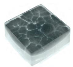
Fig. 34, Cast transparent and white soap, 7 minutes between pouring
