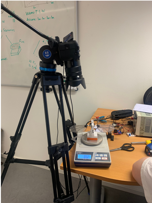
Figure 3.5: Video setup used to record the wing's stroke amplitude and frequency.
