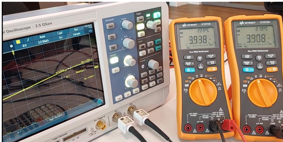
Figure 5.5: Measured induced voltage, TP4056 input voltage, and battery-side output voltage during manual operation of the generator (TP4056 output voltage).
