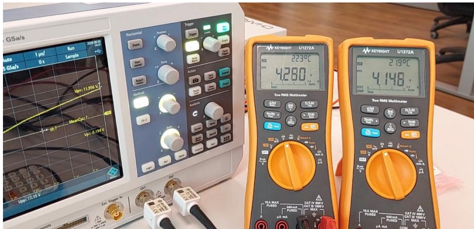
Figure 5.7: Measured induced voltage, TP4056 input voltage, and battery-side output voltage during manual operation of the generator (TP4056 output voltage).
