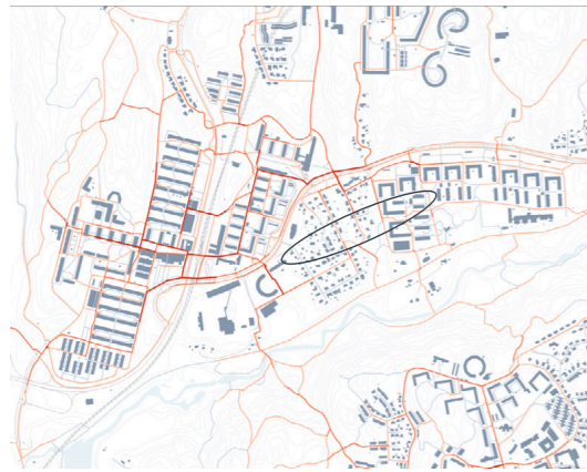
Fig. 136. Boulevard.1. Angular Betweenness 5km where sidewalks are added along Hjällbovägen and Gråbovägen in their current location.
