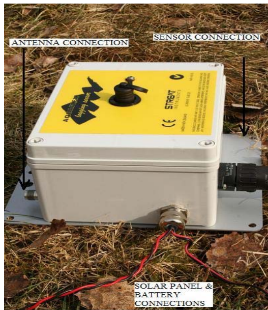
Figure 13. New Aquaflex electronic box. Lateral view. Antenna, sensor, solar panel and battery connections are visible on the picture.
