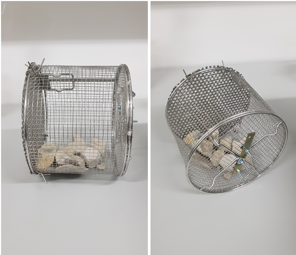
Figure 3.1: The drum constructed for the slake durability test filled with the 10 selected samples
