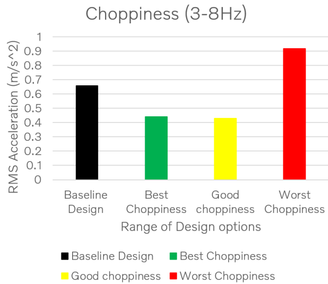
Figure 5.11: Chart indicating the seat RMS acceleration values of the ICE ride model in choppiness region for chosen design combinations
