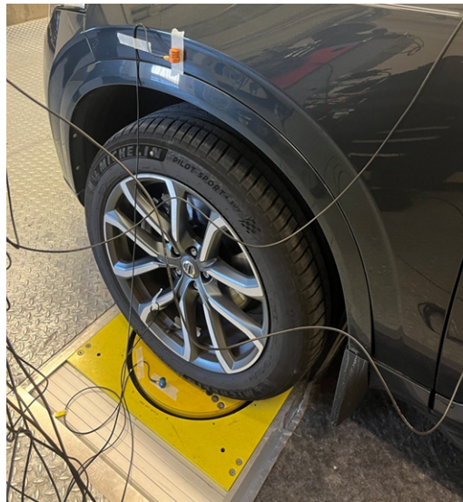
Figure 3.18: Accelerometers mounted on the skid pad, front body and front wheel
