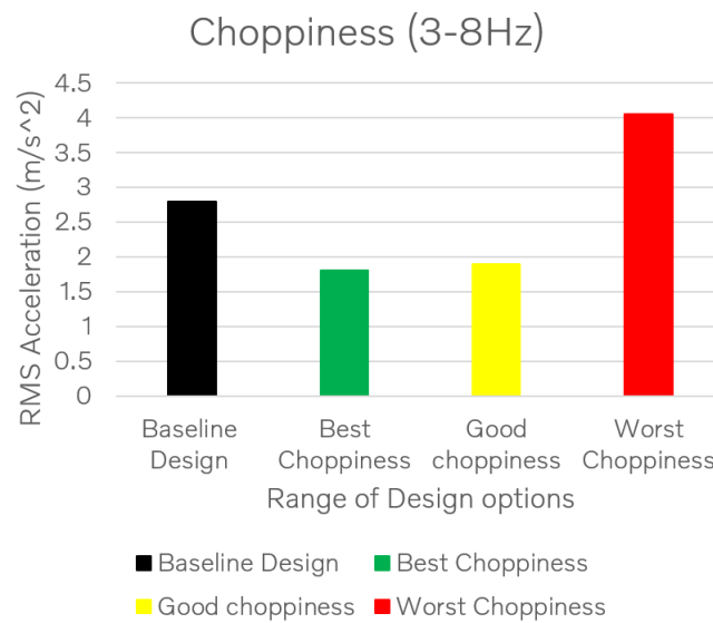
Figure 5.7: Chart indicating the seat RMS acceleration values in choppiness region for chosen design combinations with rough road as input
