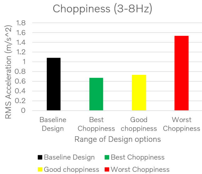
Figure 5.3: Chart indicating the seat RMS acceleration values in choppiness region for chosen design combinations
