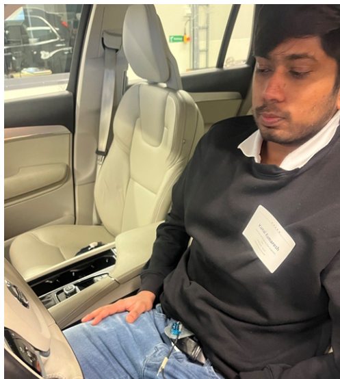
Figure 3.16: Driver with accelerometer on the belt buckle
