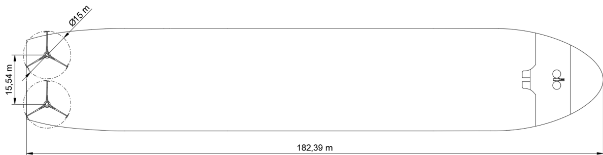
Figure 4.2: Top view of the wind power installation
