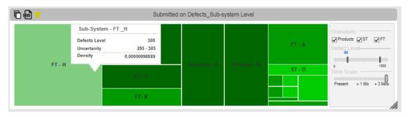
**Figure 7.4:** Defect/Density – Tree map view presenting the expected number of future defects of all the sub-systems.
