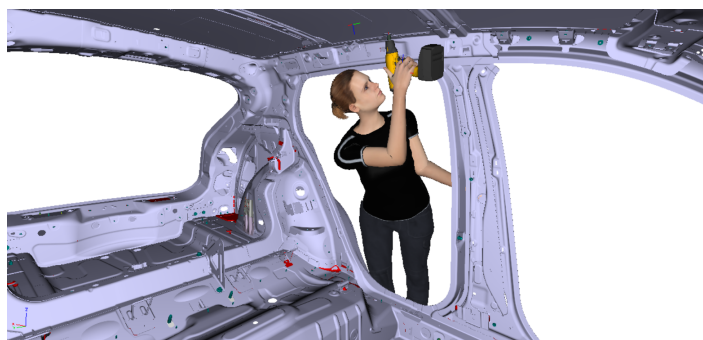
Figure 4.14: Digital illustration of how the assembly of the sunroof was performed, from IPS.
