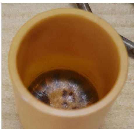
(a) Inside of crucible after \text{CrLiO}_2 solid state synthesis.
