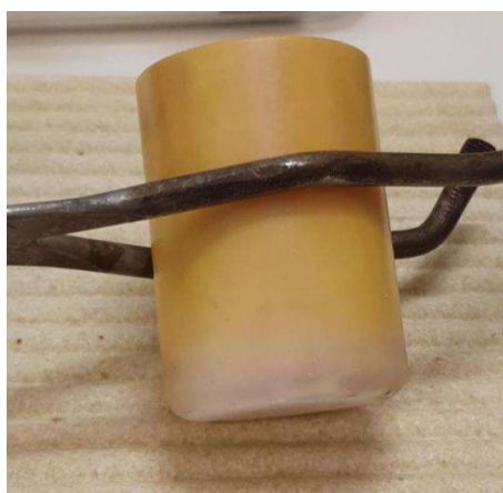
(b) Sideview of crucible after \text{CrLiO}_2 solid state synthesis. Original colour at the bottom
