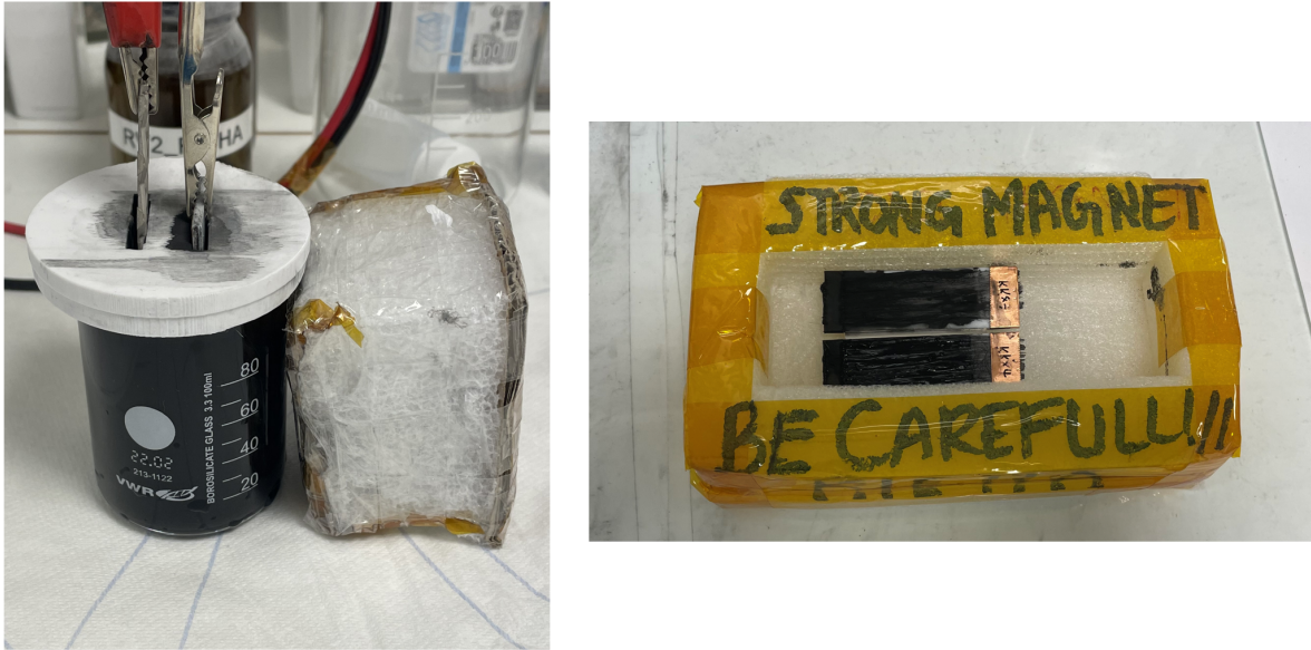
Figure 4.2: EPD Magnet Set-up: A small magnet placed adjacent to the working electrode during deposition to aid in magnetic alignment. After the deposition, the sample was dried on a large magnet for 20 minutes.
