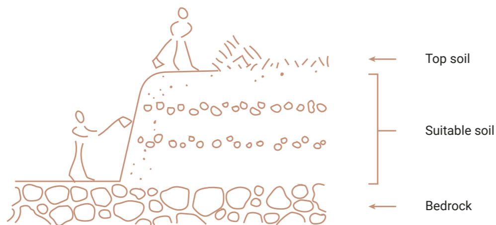
Suitable soil for construction is found in between the top soil and bedrock (Schildkamp, 2009)
