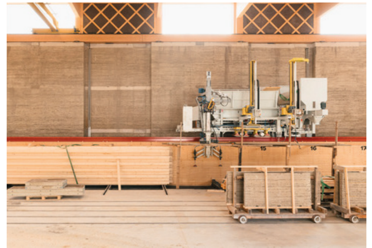
Erden's automatic rammer, feeding material and ramming up to 40 m of wall at a time and cutting elements to size (Erden, 2022)
