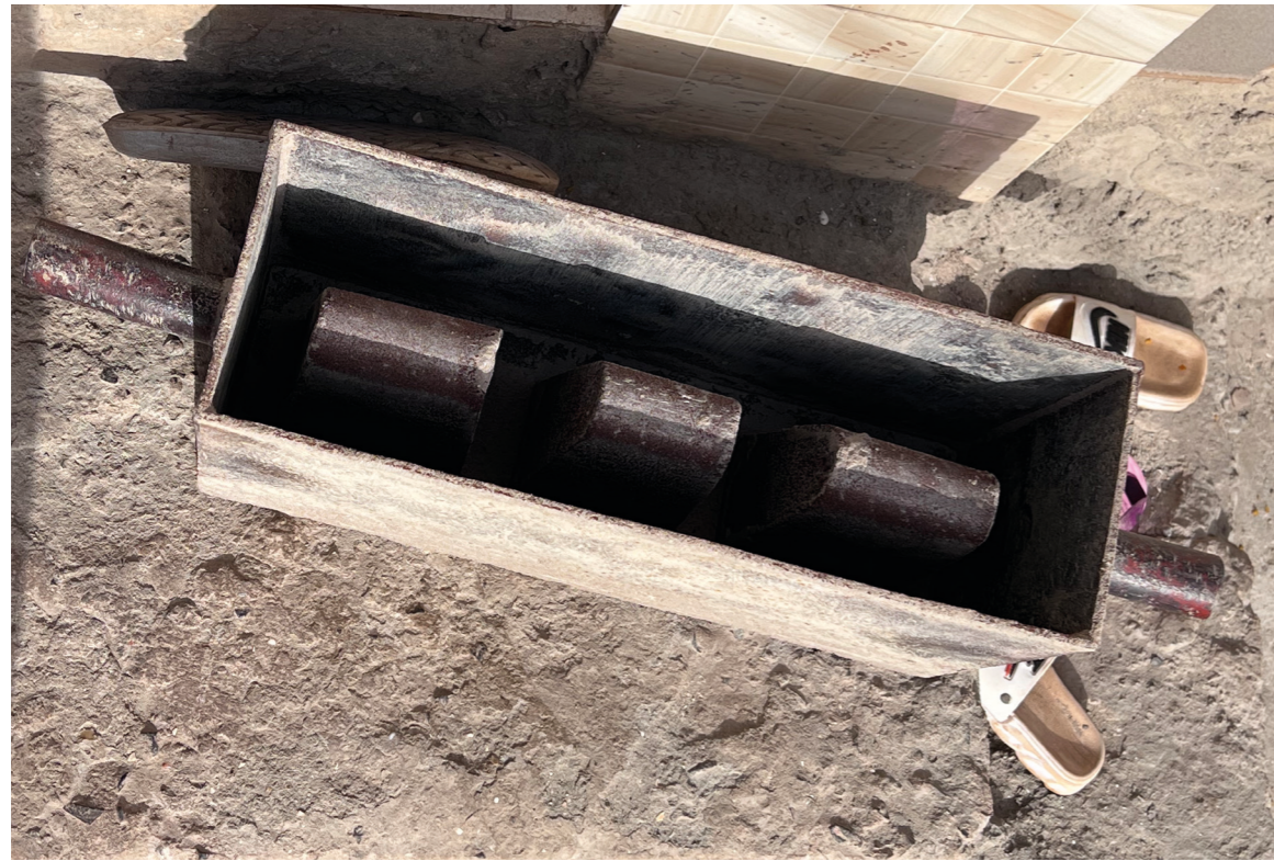
Hand-held mould for hollow concrete blocks
