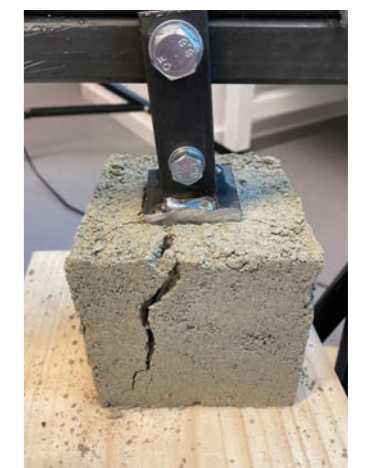
Failure of block
