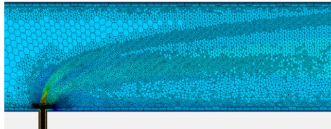
Figure 27 Adaptive mesh scene according to velocity and concentration gradient.
