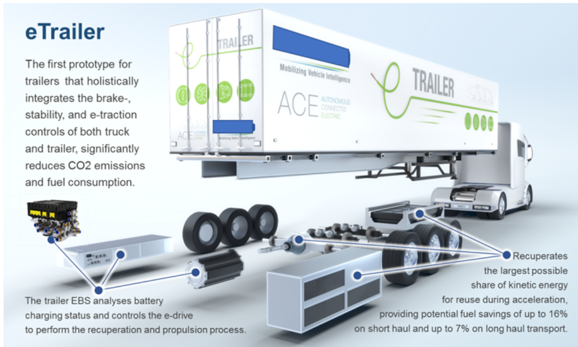
Figure 3.2: Powertrain layout and components description of ZF's E-Trailer.
