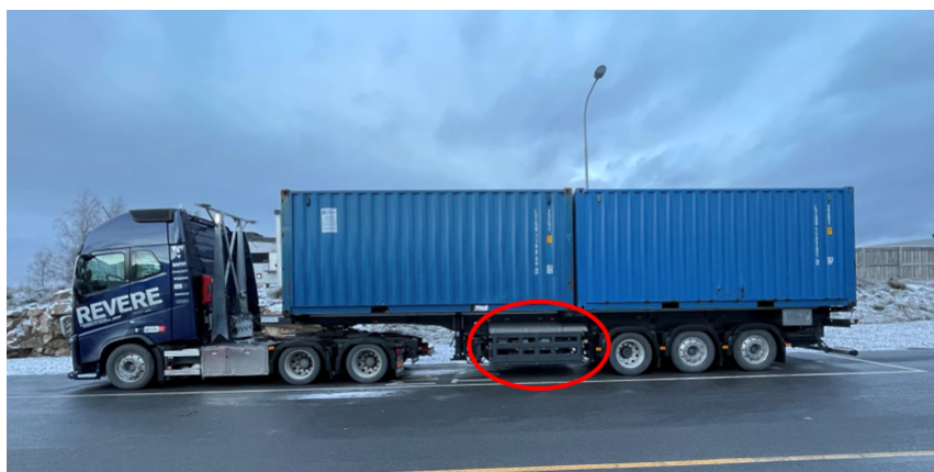
Figure 3.27: Battery position on the first generation of the E-Trailer at Volvo Trucks.
