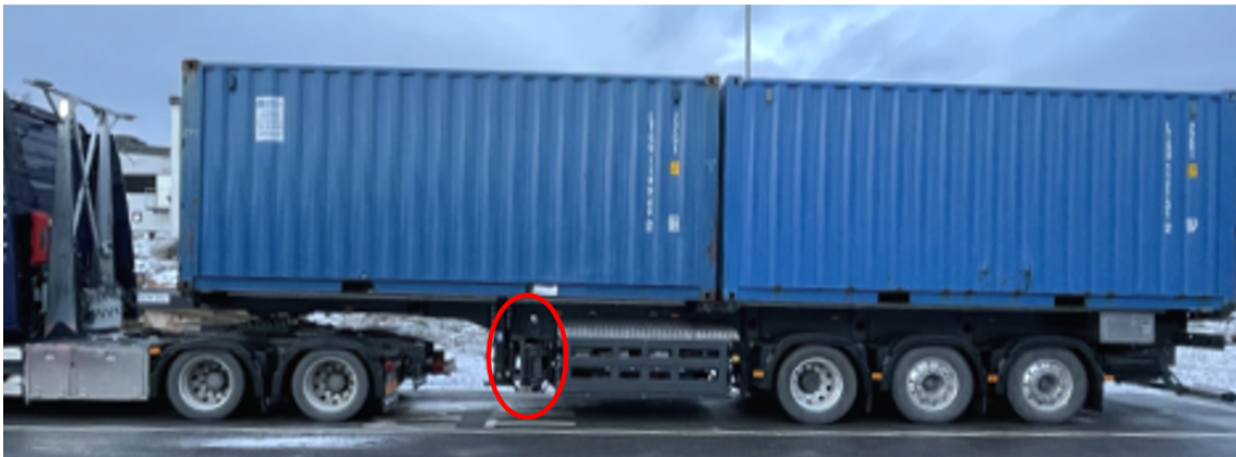
Figure 3.28: Radiator placement on the first E-Trailer
