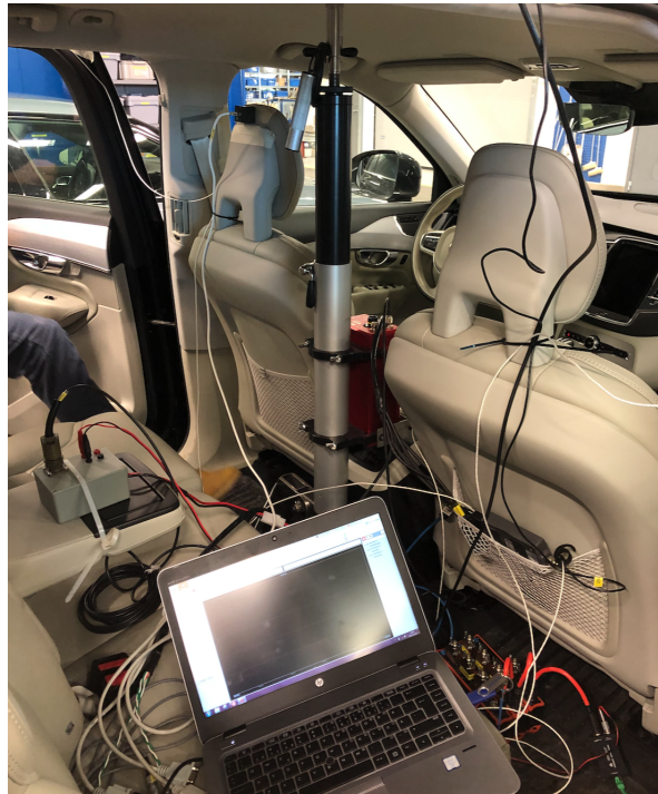
Figure 3.2: Inertial measuring unit (IMU), placed over the transmission tunnel in the car, the measuring unit itself can be seen in red between the front seats.
