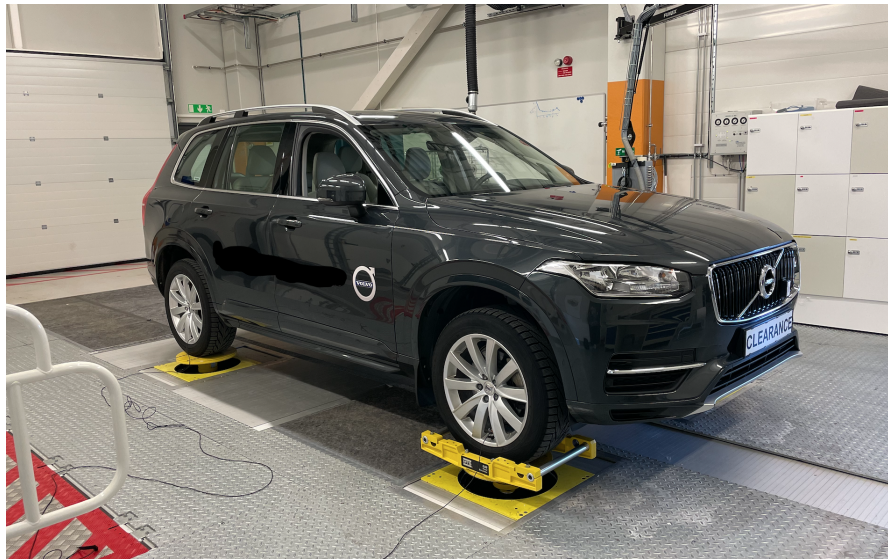
Figure 3.4: Tuning the rig to replicate physical driving by feeding sensor data from the wheels.
