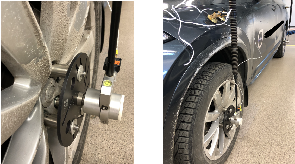
Figure 3.3: Single axis accelerometer attached to the left front wheel using a freely rotating set-up.
