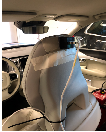
(b) Triaxial accelerometers measuring accelerations on driver seat headrest.
