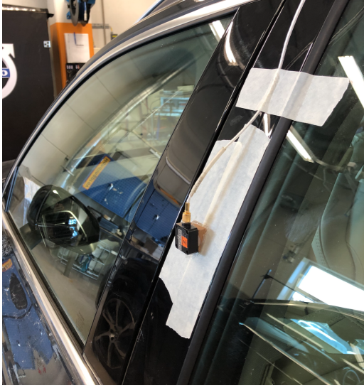
(a) Y-axis accelerometer fitted vertically on both B-pillars, pictured on the left B-pillar.
