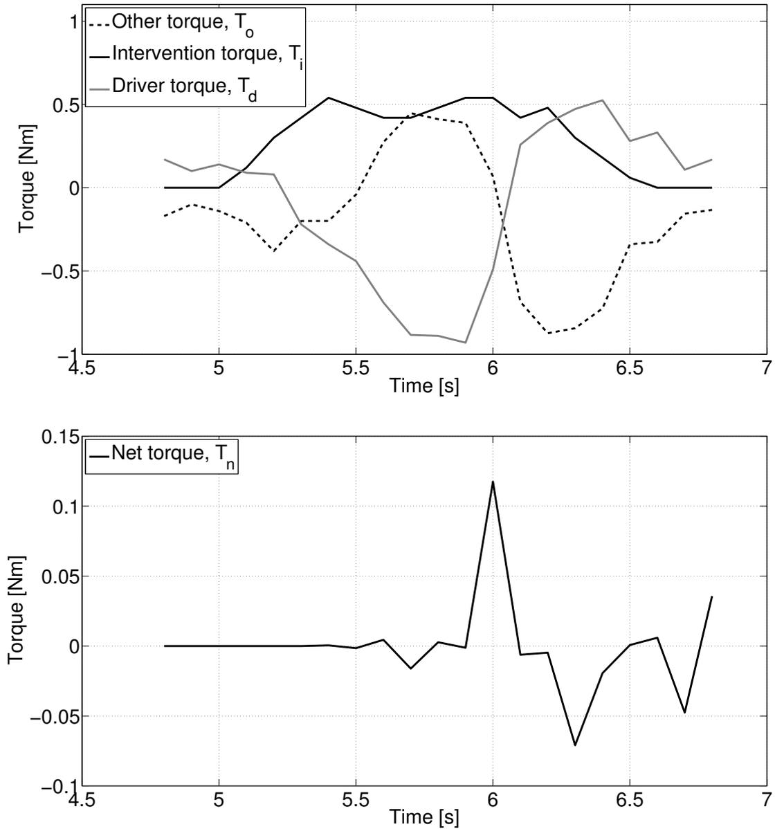
Figure 4.2: The other torque, intervention torque, driver torque, and net torque during an intervention. The intervention starts at 5.0s and ends at 6.6s, and the event has the DIT rate of  $8.7 \text{ N m s}^{-1}$ .
