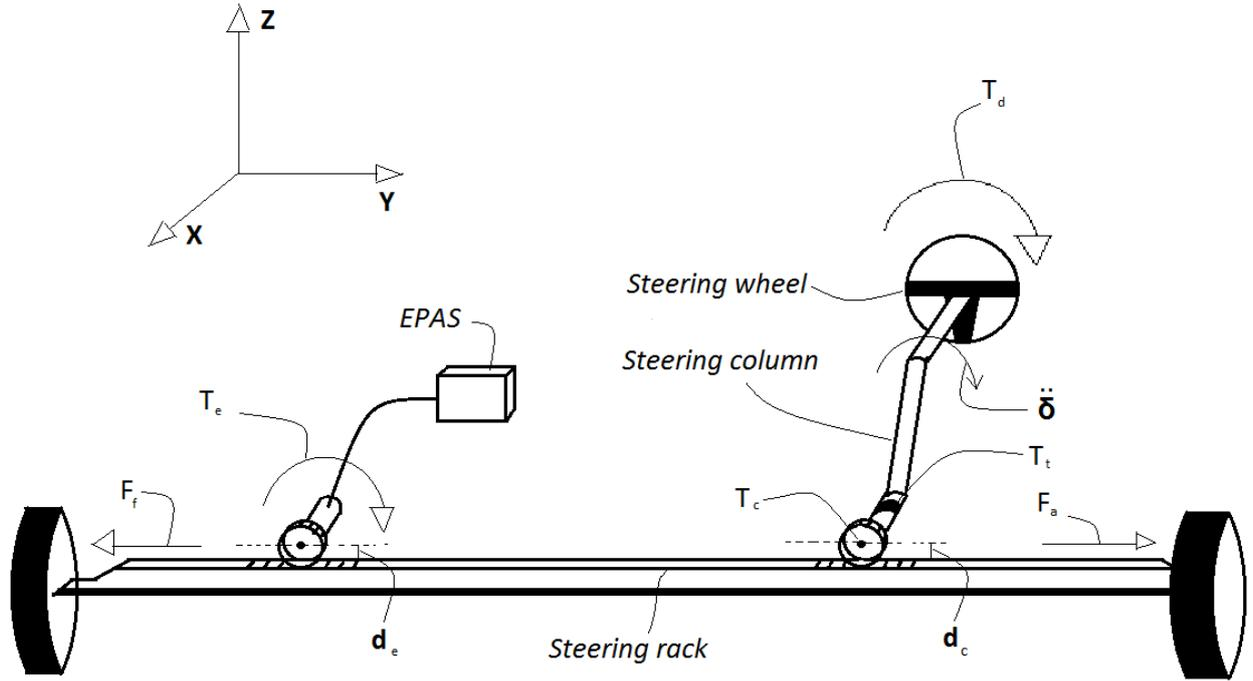
Figure 2.3: Sketch over the whole steering arrangement with the EPAS, steering rack, steering column, steering wheel, and all the torques  $T$ , distances  $d$ , and forces  $F$  that exist in the system of interest.
