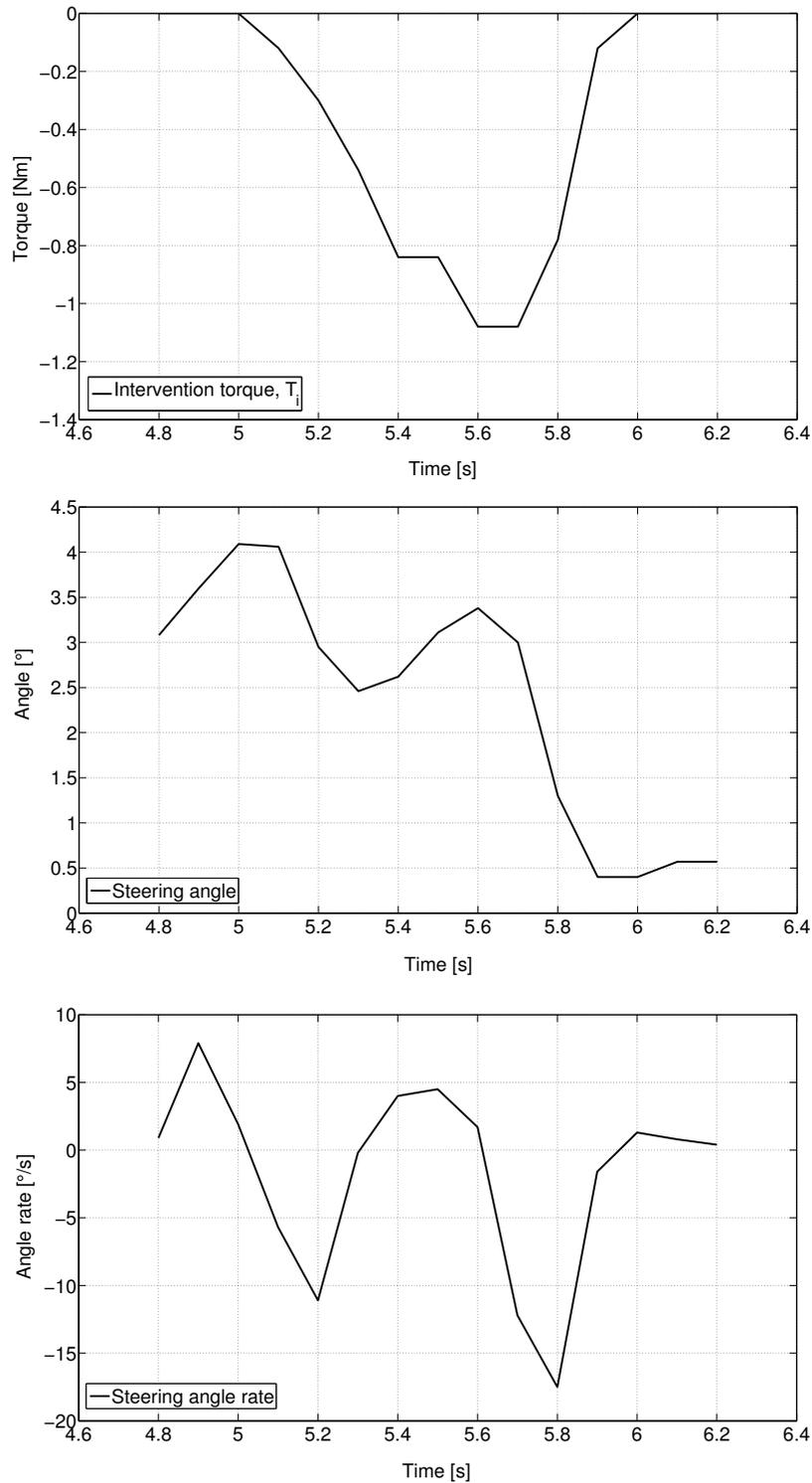
Figure 4.4: The intervention torque, the steering wheel angle and its rate value for an intervention. The intervention starts at 5.0s and ends at 6.0s, and the event has the DIT rate of  $13.5 \text{ Nm s}^{-1}$ .
