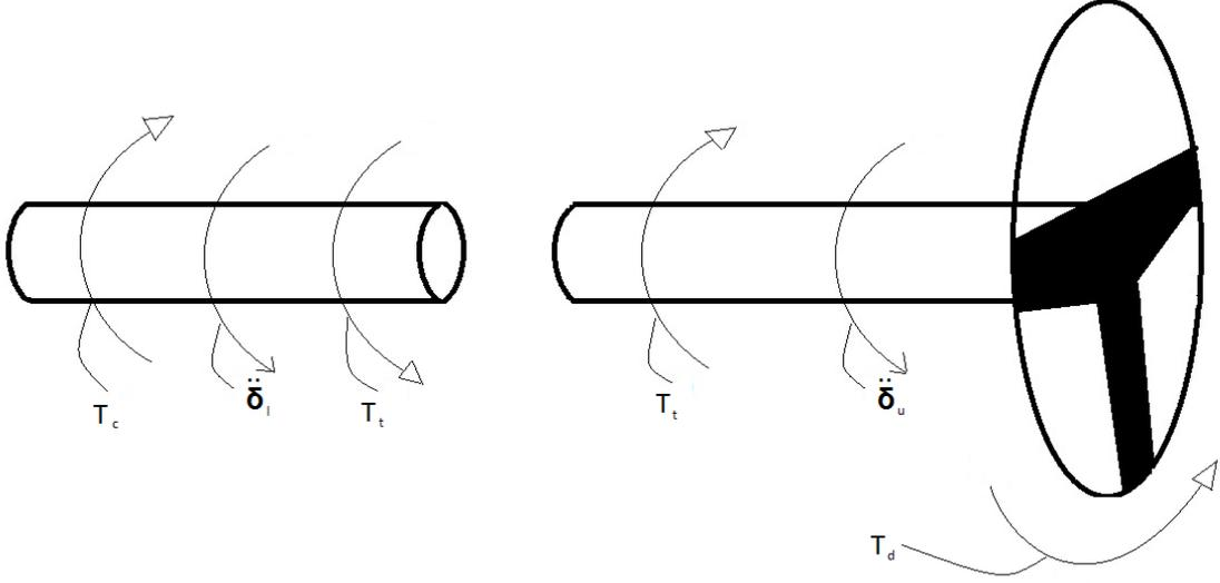
Figure 2.4: The *free-body sketch* as an approximation of the steering arrangement, with all the torques and movement terms.
