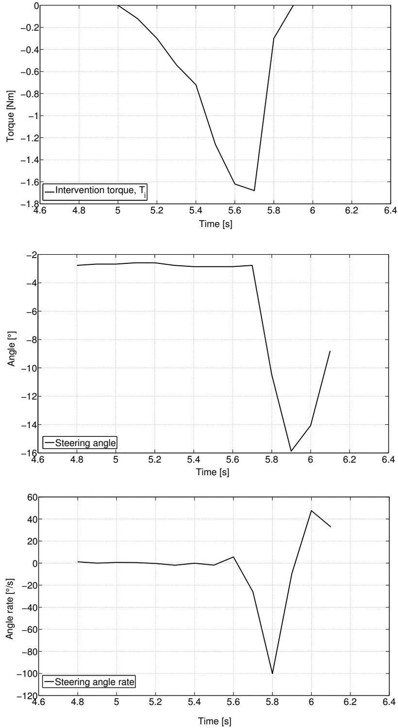
Figure 4.6: The intervention torque, the steering wheel angle and its rate value for an intervention. The intervention starts at 5.0s and ends at 5.9s, and the event has the DIT rate of  $42.0 \text{ Nm s}^{-1}$ .
