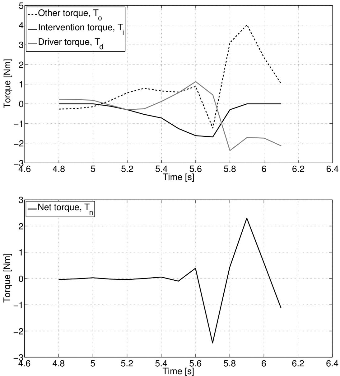
Figure 4.3: The other torque, intervention torque, driver torque, and net torque during an intervention. The intervention starts at 5.0s and ends at 5.9s, and the event has the DIT rate of  $42.0 \text{ N m s}^{-1}$ .
