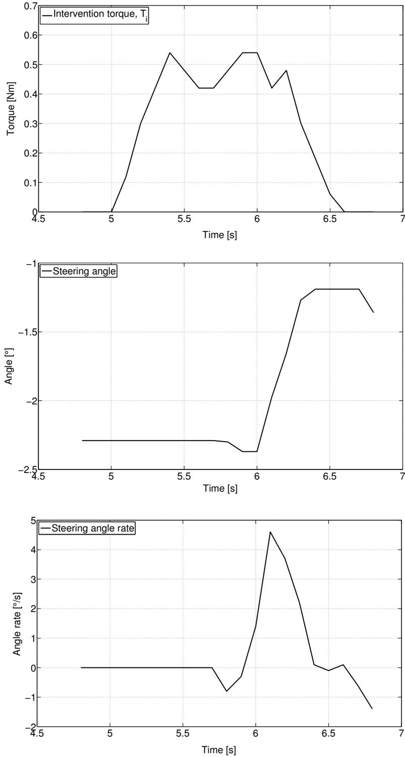
Figure 4.5: The intervention torque, the steering wheel angle and its rate value for an intervention. The intervention starts at 5.0s and ends at 6.6s, and the event has the DIT rate of  $8.7 \text{ N m s}^{-1}$ .
