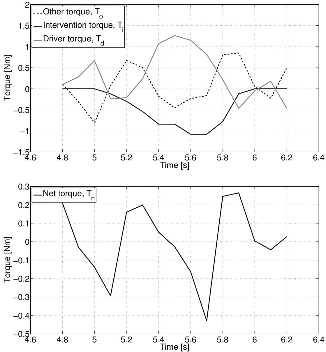
Figure 4.1: The other torque, intervention torque, driver torque, and net torque during an intervention. The intervention starts at 5.0s and ends at 6.0s, and the event has the DIT rate of  $13.5 \text{ N m s}^{-1}$ .
