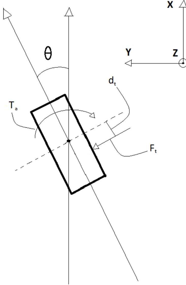
Figure 2.2: Sketch over the origin of the  $T_a$ , seen from a top view over a front wheel. The  $T_a$  originates from the distance  $d_t$  to the  $F_t$ . The car is travelling in the x-direction and the wheel is pointing in an offset direction with an angle  $\Theta$ .
