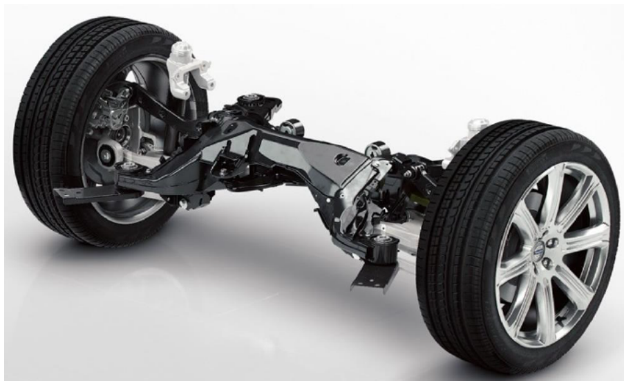
Figure 2.6: Integral link suspension from a Volvo XC90 [5]
