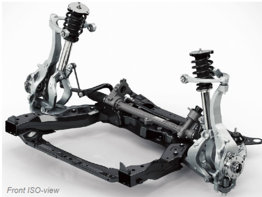
Figure 2.5: Short Long Arm suspension from a Volvo XC90 [5]
