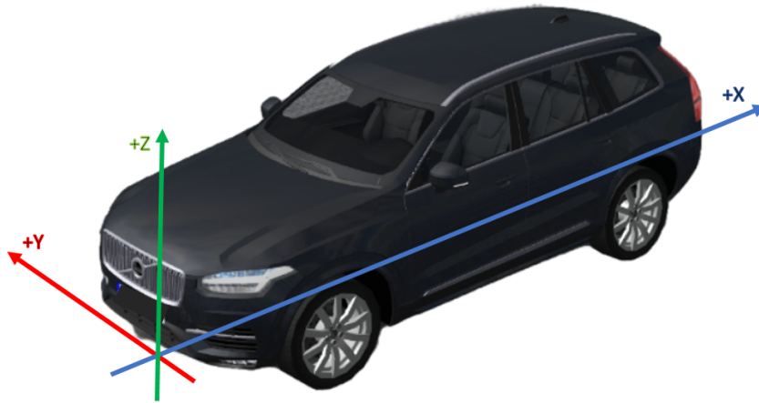
Figure 2.7: Illustration of axis system used in vehicle design
