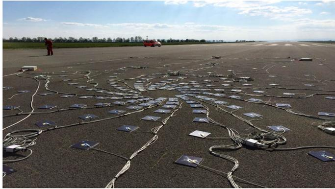
**Figure 1.2:** The microphone array located at the Magdeburg-Cochstedt private airfield
