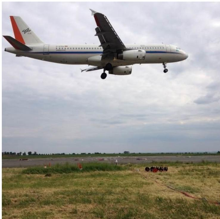
**Figure 1.1:** The research aircraft of DLR flying above the microphone array
