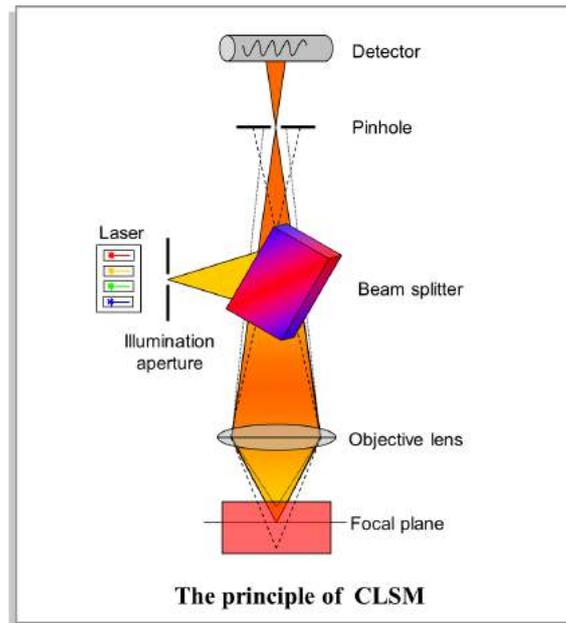
**Figure 2.6:** Schematic set up CLSM. Image courtesy of Annika Altskär, RISE.
