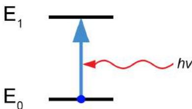
**Figure 2.5:** Excitation of an atom or a molecule when absorbing energy ( $h\nu$ ). The atom or molecule excites from ground state,  $E_0$ , to the next level of energy,  $E_1$ , also referred to as the excited state.
