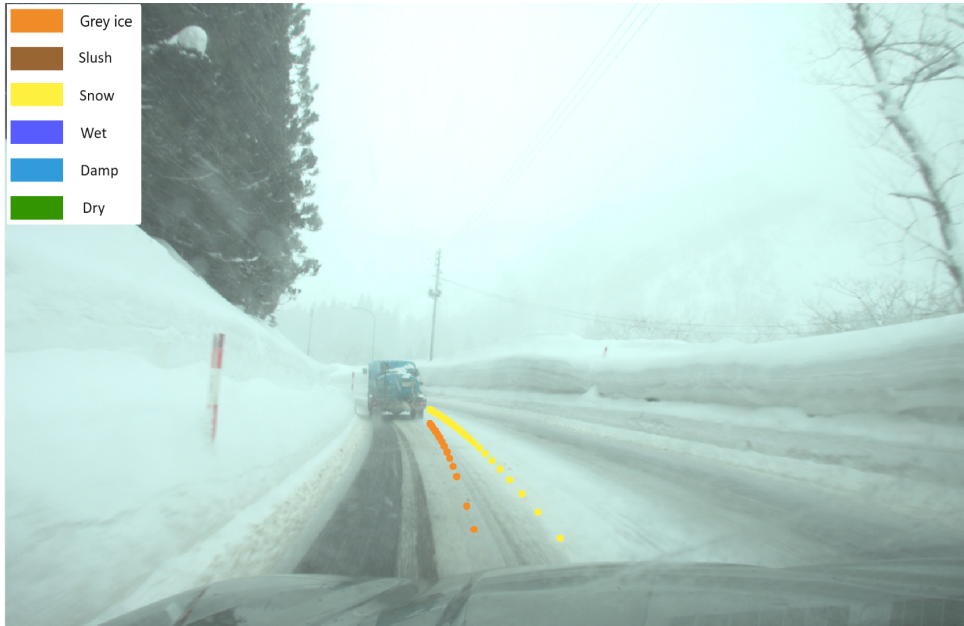
Figure 3.1: RSC Determined by the Lasers During a Vehicle Ride. Showing coloured dots representing the points on the road surface where the lasers have performed measurements. For each measured point, the colour corresponds to the RSC determined by the laser. The legend in the top left corner describes the specific RSC categories and their respective colour.
