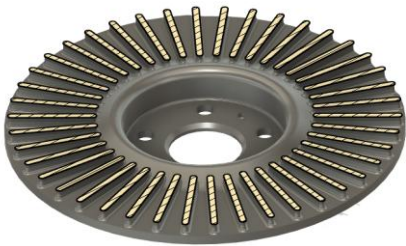
Figure 12: Ventilation layer in 3D model
