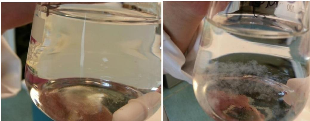
Figure 4.6 a) The picture to the left shows magnesium silicate with inhibitor P5, b) The picture to the right shows magnesium silicate without inhibitor.
