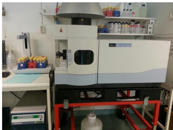
Figure 3.1: ICP-MS instrument
