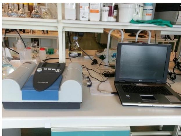
Figure 3.2: Schematic of UV-VIS apparatus
