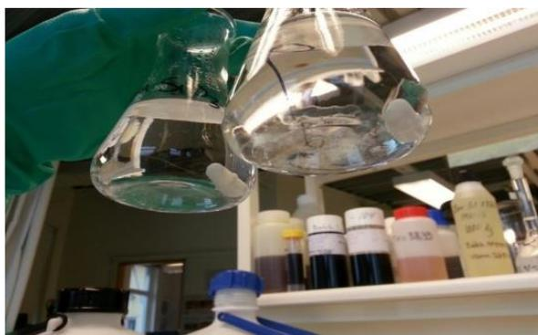
Figure 4.2: Flask to the left is calcium silicate and flask to the right is magnesium silicate at  $90^\circ\text{C}$  (pH=8.0)
