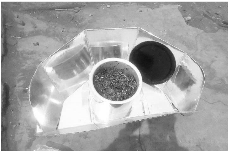
Figure 4.2 The panel solar cooker called CookKit.
