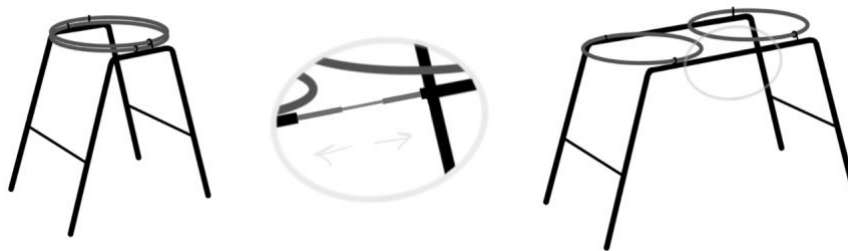
Figure 11.2 Far left shows the stand in its original state, the illustration in the middle shows how the stand is extendable and far right shows the stand in its extended state.
