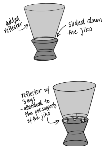
Figure 10.2 Combining the solar cooker with the jiko stove.
