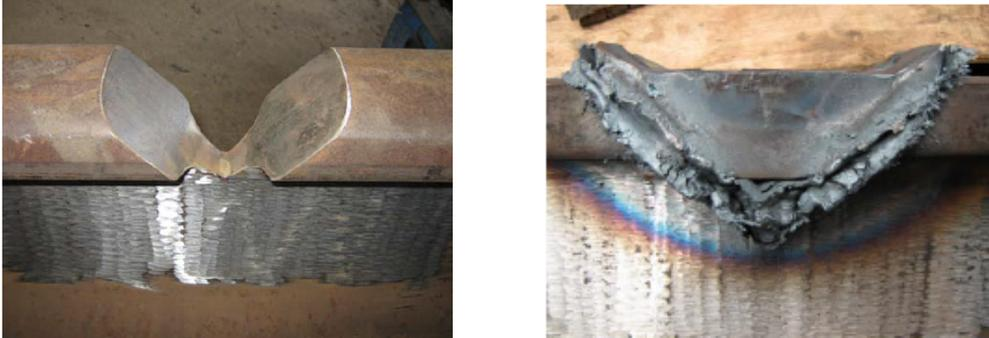
Figure 1.2 – Carved slot (left) and completed flash butt weld (right) [8]
