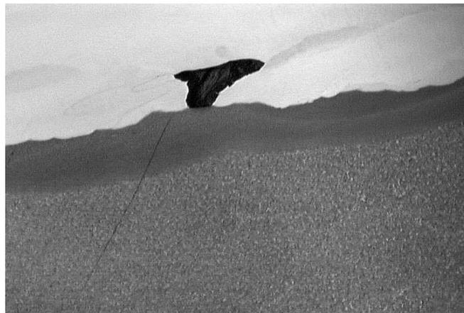
Figure 2.1 – Fatigue initiation feature in a MMA weld repair of rail [5]
