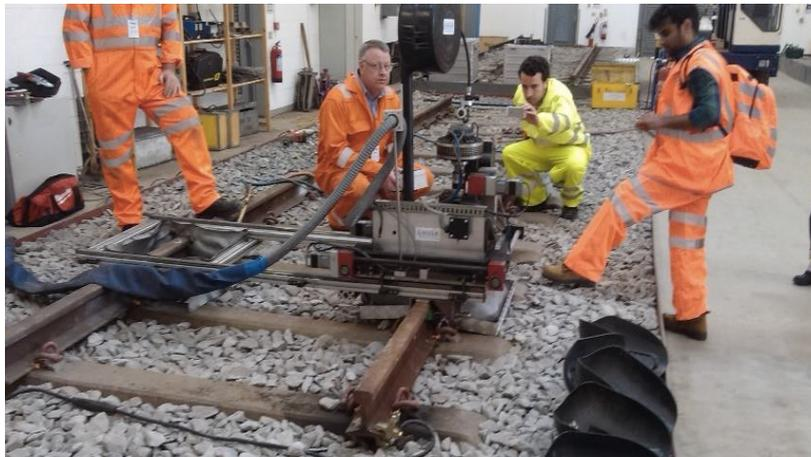
Figure 1.5 – Prototype unit employed during the DDR tests [10]
