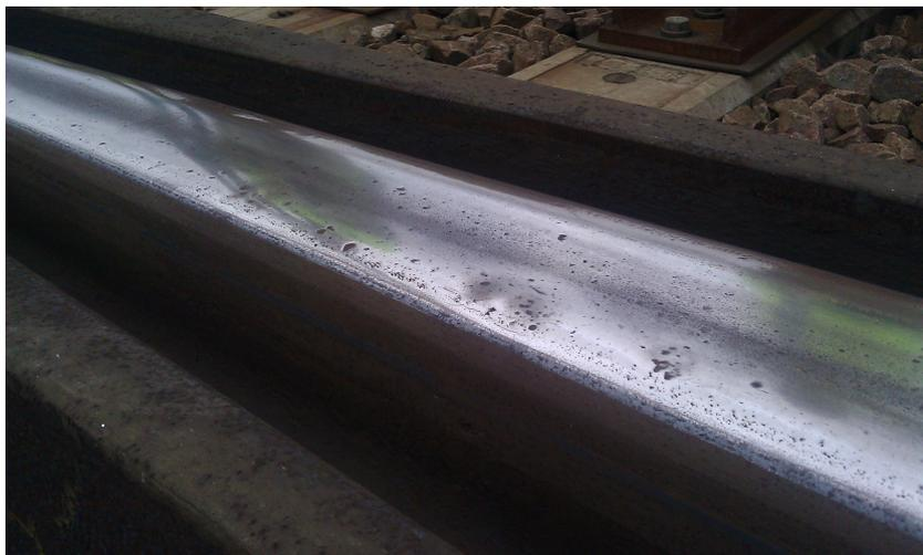
*Figure 1.1 – Rail surface affected by squats (picture courtesy A. Ekberg)*
