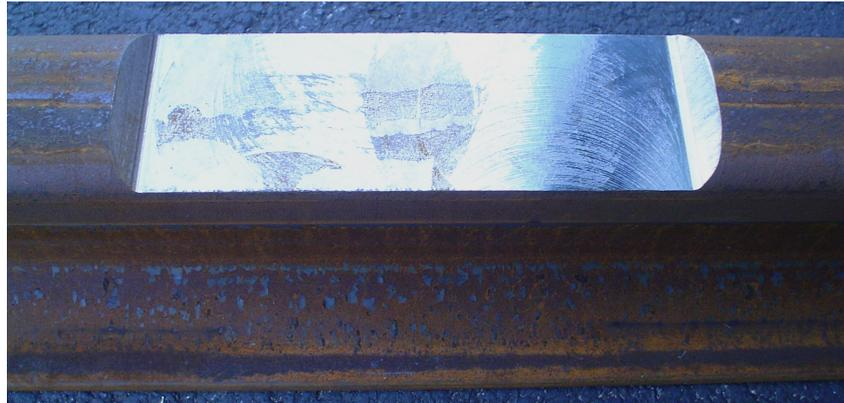
Figure 1.4 – Milled cavity [7]
