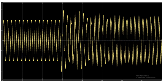
Figure 2.2: Bus voltage: 0p.u. , capacitor voltage: 0p.u. , giving a voltage difference \Delta = 0p.u. between bus and capacitor. Transient voltage is detected, but not at extreme levels.
