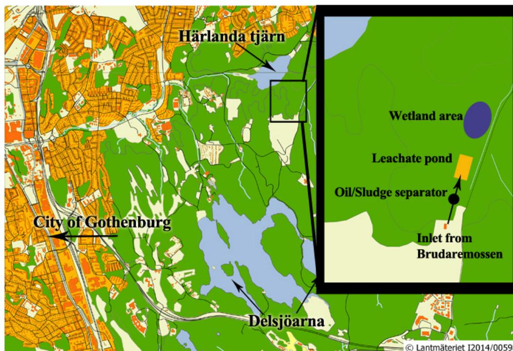
Figure 6.3 The existing treatment of landfill leachates; oil and sludge separator followed by a leachate pond and wetland area situated to the north of Brudaremossen [background map from (Lantmäteriet, 2014)].
