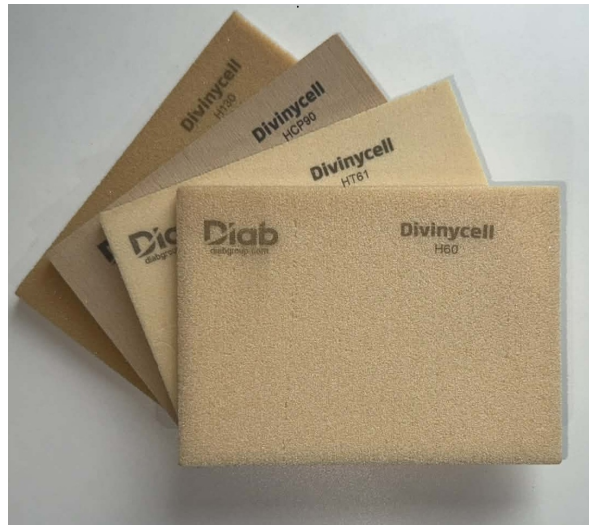
Figure 1.2: Foams core samples of different grades and categories.
