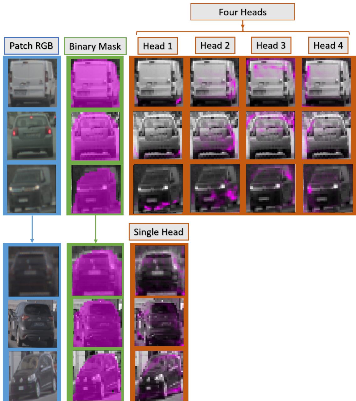
Figure 5.3: Visualization of binary mask and attention masks for AHA experiments. Stronger pink colour in a pixel indicates large weight in the mask. Here, masks from AHA 1H and AHA 4H are shown, to compare how number of attention heads affects mask interpretability.
