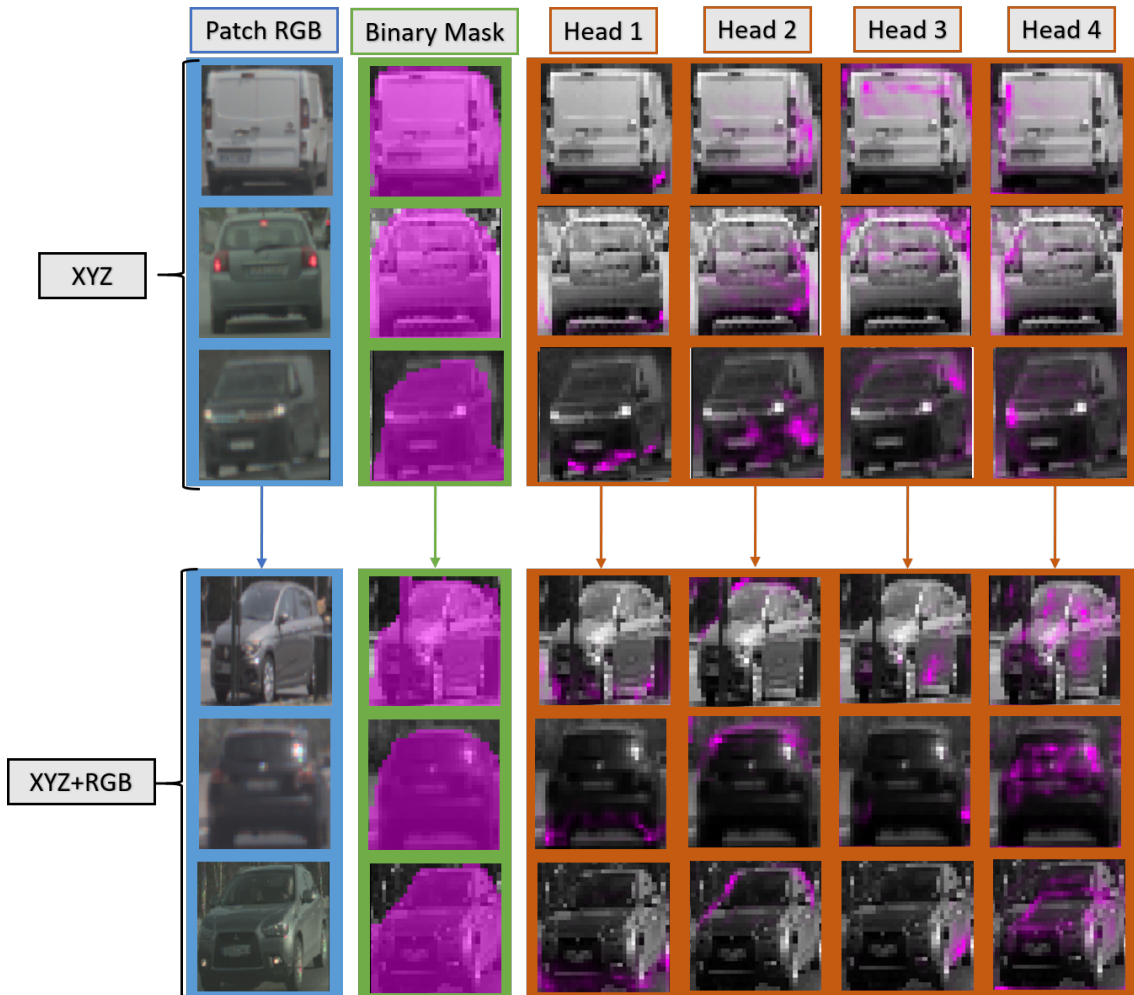
Figure 5.4: Visualization of binary mask and attention masks for AIA experiments. Stronger pink colour in a pixel indicates large weight in the mask. Here, masks from AIA XYZ and AHA RGB are shown, to compare how number of attention heads affects mask interpretability.
