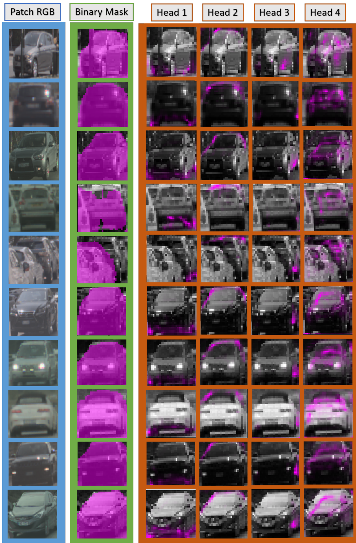
Figure 5.1: Visualization of binary mask and the four attention masks for AIA RGB, for non-occluded objects. Stronger pink colour in a pixel indicates large weight in the mask.
