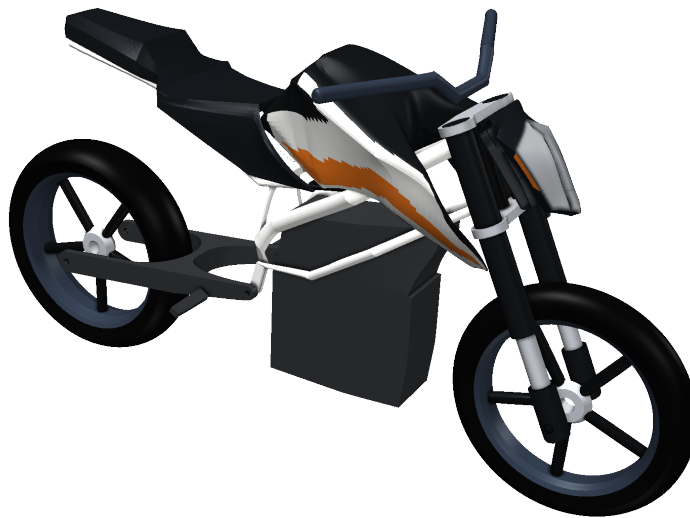
Figure 4.32: Representative FE-model of the KTM Duke 390.
