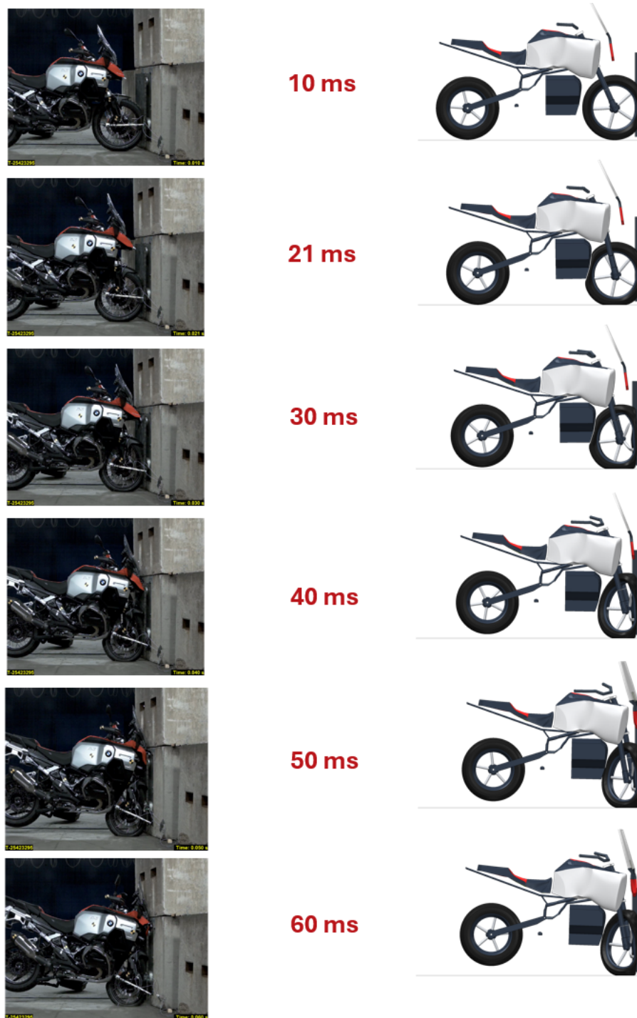
Figure 4.58: Side by side comparison between the physical crash test and the simulation at selected time stamps, BMW GS1300.
