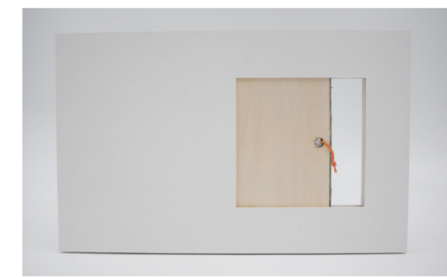
(6) Early physical model of a hatch. Here it is completely integrated into the wall, something we eventually decided against for acoustical reasons.
