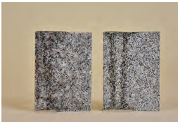
Fig 3.33 Investigation of the stone when wet
