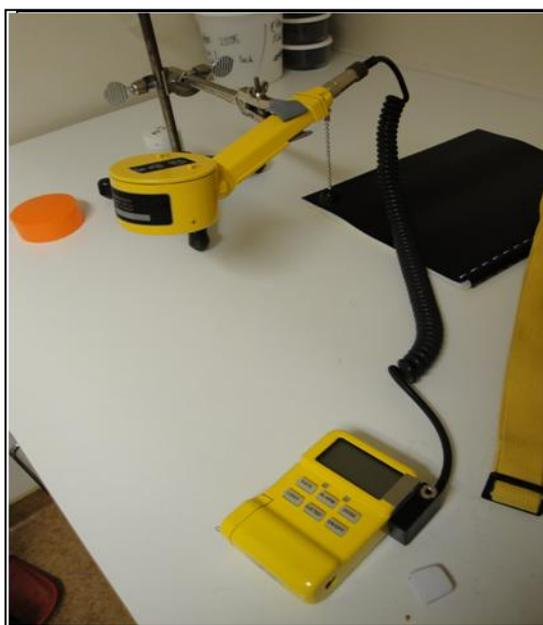
Viability for surgical uses of a portable NaI(Tl) scintillator detector.
