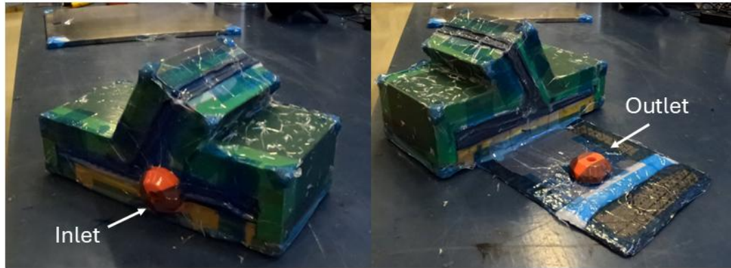
Figure 18: Resin inlet and outlet shown on a mould after the part has cured and the bag removed.
