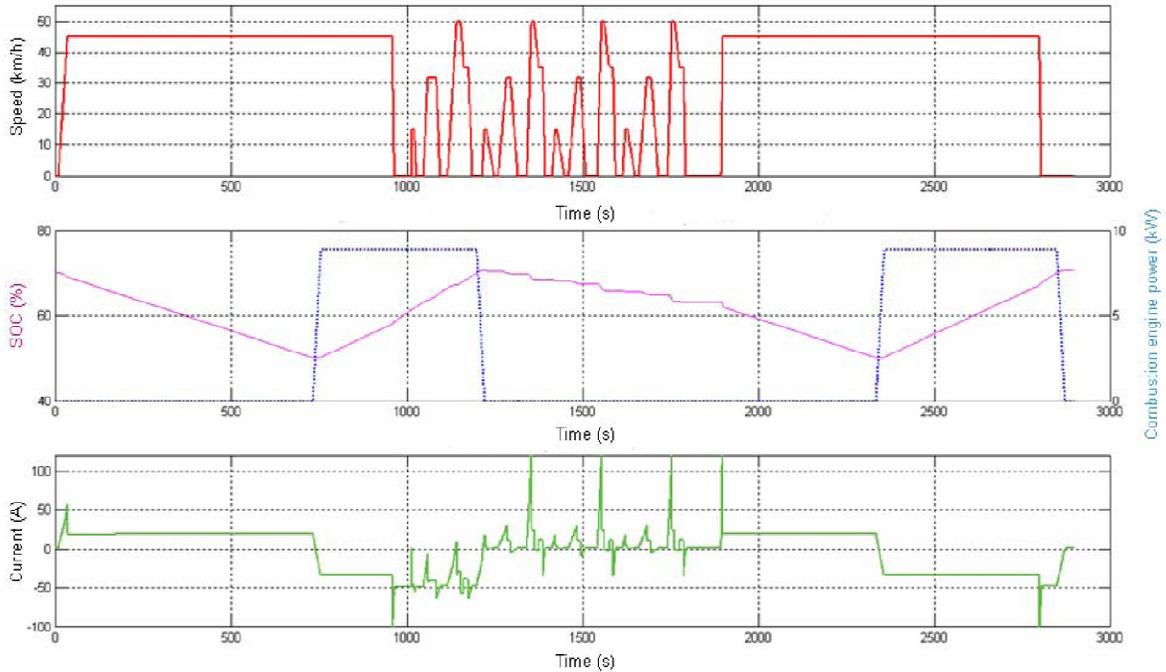
Fig.3. 18 Speed variation and current drawn from the battery by the Electric motor. With regenerative breaks SOC can fall more slowly. By courtesy of Dr. Felipe Jimenez , EPISOL project ,Polytechnic University of Madrid (UPM)
