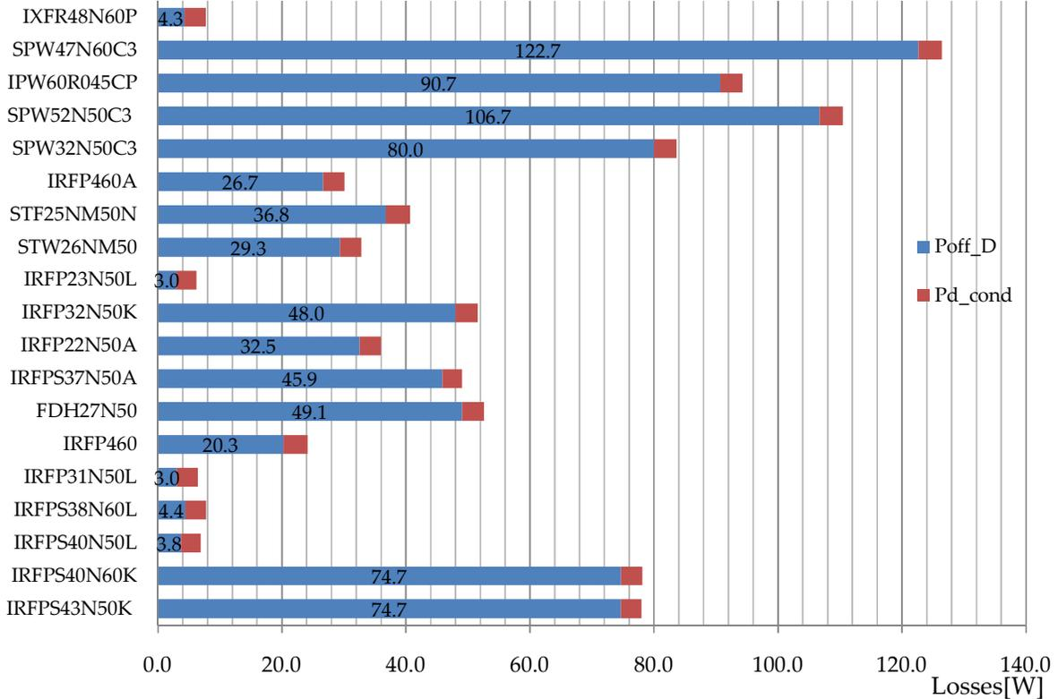
Fig.5. 11 conduction losses and turn-off losses of diode in secondary side, the sum will be total secondary losses. (Pout=3600W) Switching losses based on  $I_{con} = 1.2A$  for all switches (simplified model)
