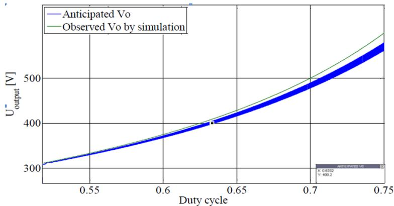
Fig.8. 3 Open loop performance of fullbridge boost DC-DC converter in a range of duty cycles ; The observed output voltage diverges from anticipated output voltage esp. At higher duty cycles.
