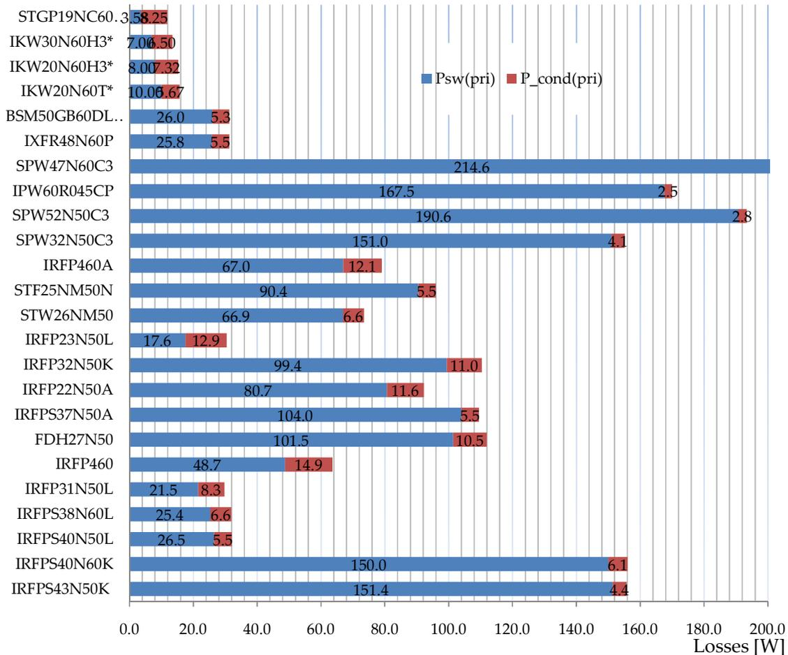
Fig.5. 10 Primary side, switching losses (Switch turn-on and off) and Conduction losses for a single switch (\* represents IGBTs) (Pout=3600W). Switching losses based on  $I_{Gon} = 1.2A$  for all switches(simplified model)
