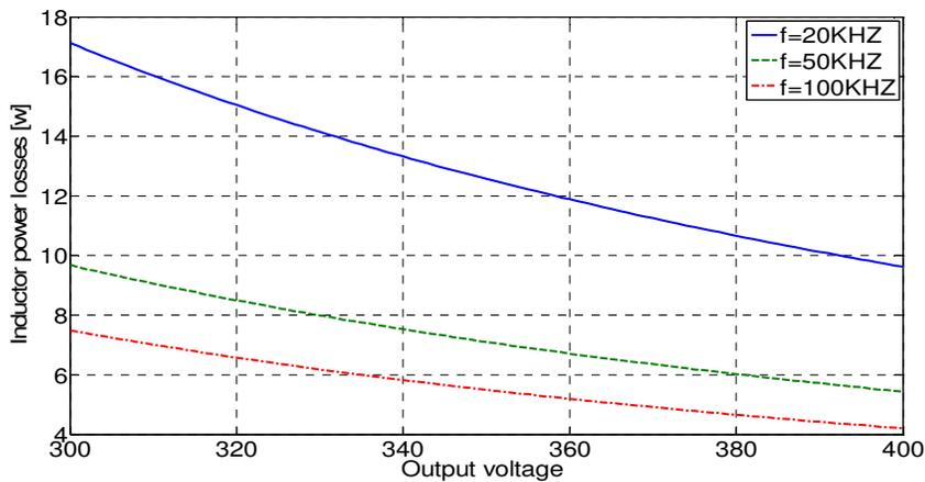
Fig.6. 4 Total inductor losses as a function of output voltage in 3 different frequencies (Core: *E713332E250*, Airgap: 5.28mm) at  $P_{out} = 3600W$
