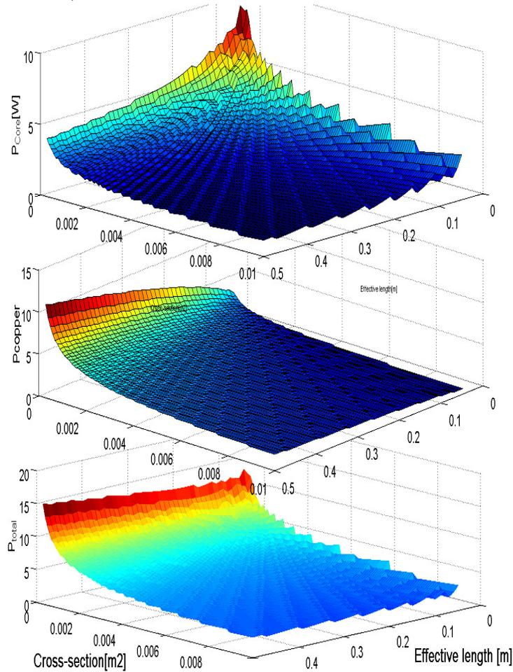
Fig.6. 2 Inductor losses vs. Cross-section and Effective length, for  $L_{ind} = 0.0037 H$ , Material: 3C90
