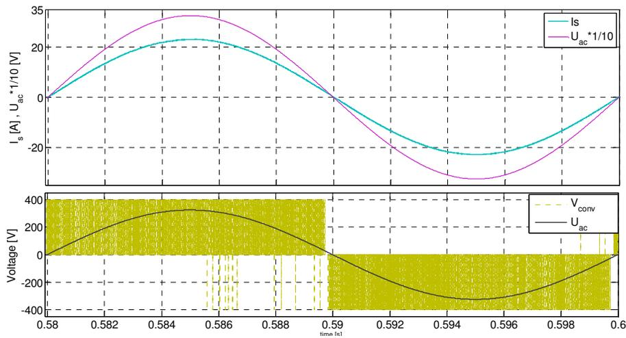
Fig.9. 7 (up) Output current  $i_s$  and grid voltage.  $I_s$  is sinusoidal, but  $180^\circ$  behind the voltage but for comparing it is multiplied by -1 here, also grid voltage is 0.1 of its real value. (down) PWM unipolar switching pattern
