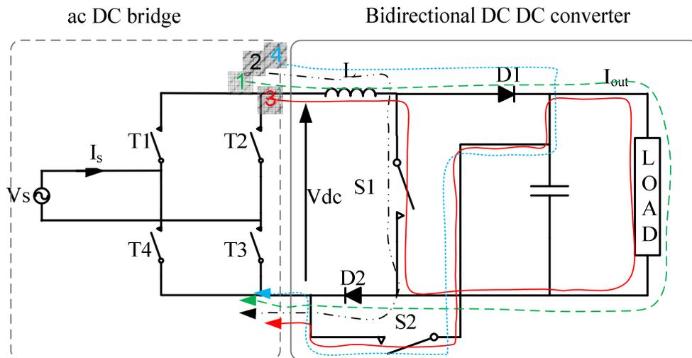
Fig.2. 1 a Bidirectional ac-DC converter topology
