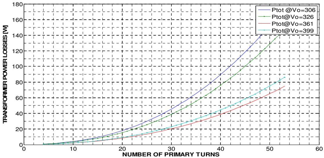
Fig.B. 4 Transformer total losses as a function of number of primary turns when the core is EC70 ( $airgap = 1830 \mu M, \mu r_{3F3} = 2000$ ) (linear scale)
