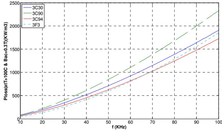
Fig.4. 14 core losses as a function of frequency (sine wave)
