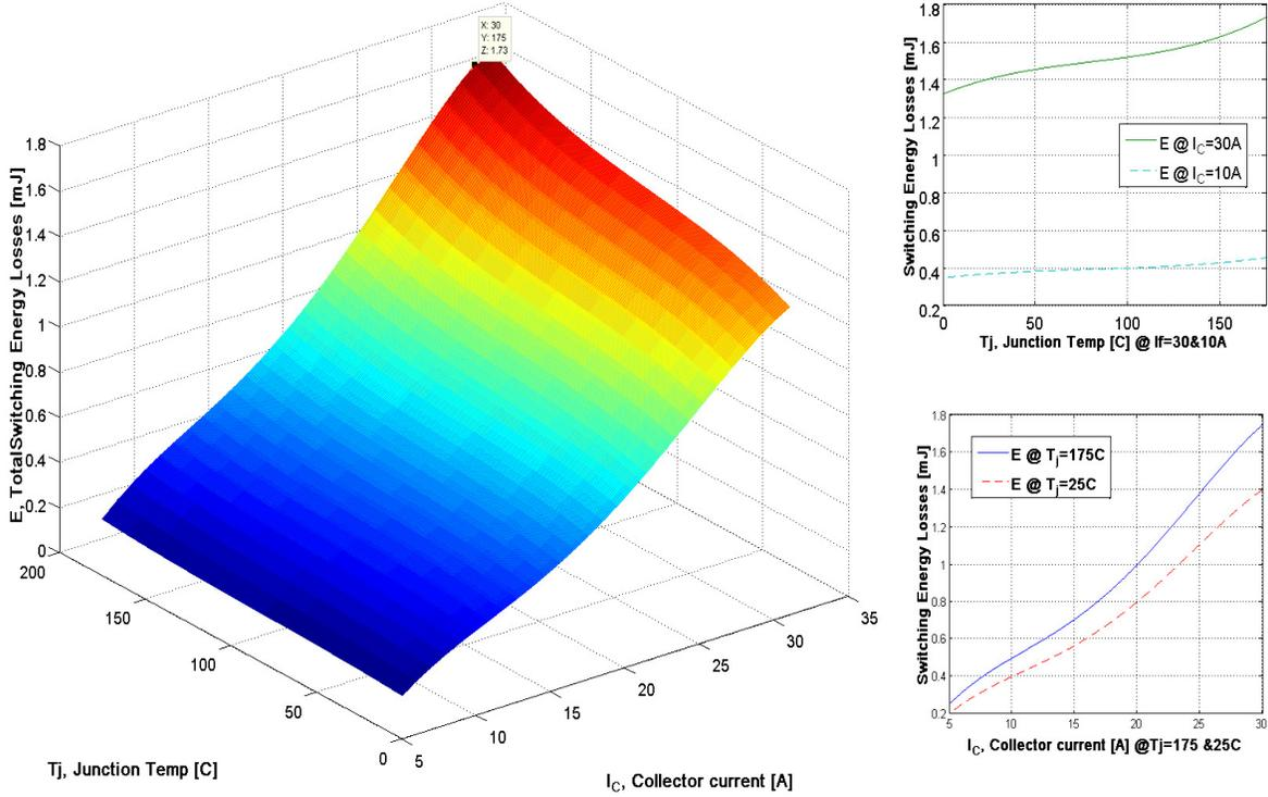
Fig.5. 7 Total switching energy losses as a function of collector current and temperature for the “IKW30N60H3” IGBT at  $R_G = 10.5$
