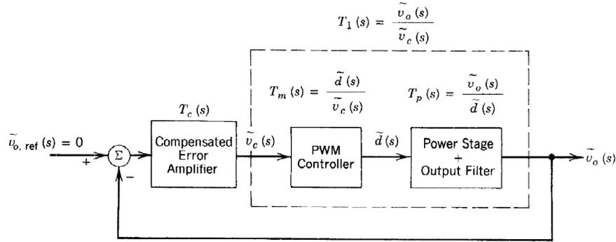
Fig.8. 7 Closed loop block diagram
