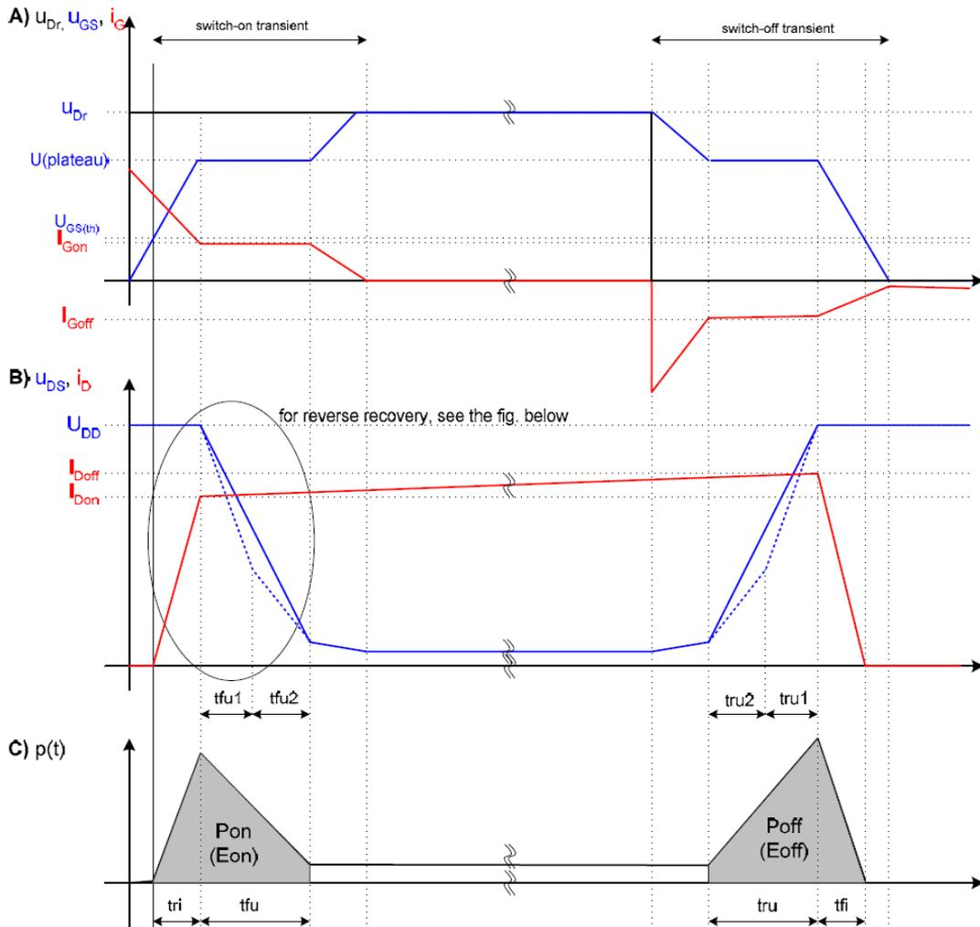
Fig.4. 5 Switching turn-on and turn-off transient and Losses of a MOSFET (without considering Reverse recovery)
