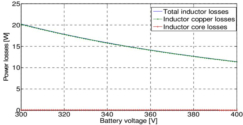
Fig.7. 3 Inductor losses as a function of battery voltage (Core: E713332E250, Airgap: 5.28mm) at  $P_{bat} = 4000W$  and  $f_{sw} = 20kHz$  (core losses are close to zero)
