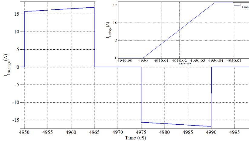
Fig.6. 5 Transformer current (flux density) waveform and the switching transient (leakage=1uH)
