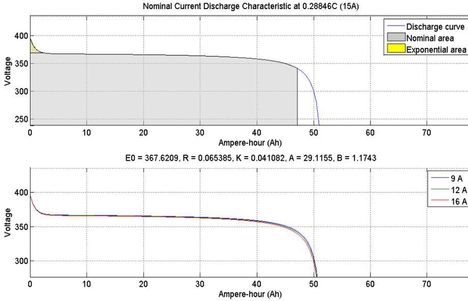
Fig.3. 16 The battery discharge characteristics for 3 different discharge current (9A, 12A, 16A). The gray Area depicts the extractable battery energy (which we chose to be around  $17kWh$ , this value is less than total battery energy). Charge characteristics will be the opposite if we neglect the hysteresis effect of the battery
