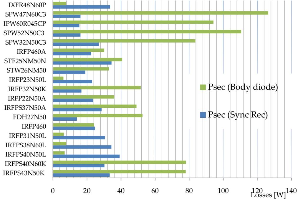
Fig.5. 22 comparison of synchronous rectification switch losses and body diode losses in the secondary side, for a DC-DC full-bridge converter (output power:3.6 KW)
