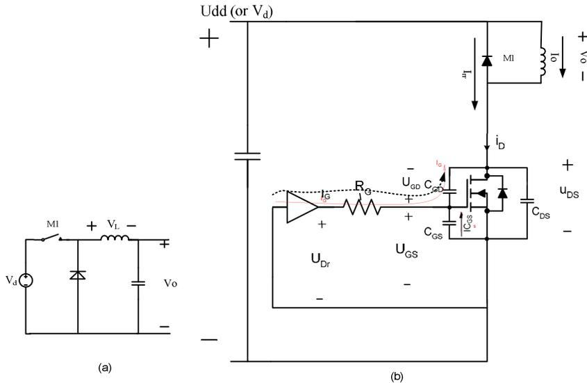
Fig.4. 4 a) Conventional Buck converter. b) The equivalent dynamic test circuit, suitable for studying the transient analysis and the role of body diode, M1, note that we assume  $I_o = cte$  for all the times.
