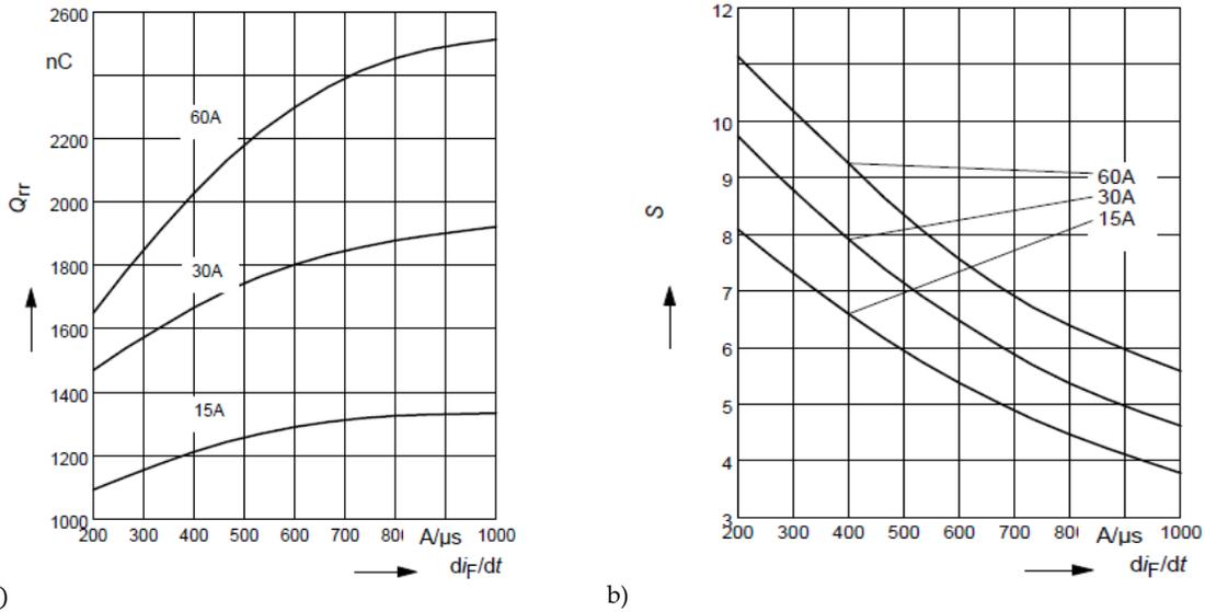
Fig.5. 16  $Q_{rr}$  and  $S$  as a function of  $di_F/dt$  for IDB30E60. Courtesy of infineon ([www.infineon.com](http://www.infineon.com)) Addition to  $S$  and  $Q_{rr}$ ,  $I_{rr}$  and  $t_{rr}$  are also affected by  $di_F/dt$ . By increasing  $di_F/dt$ ,  $I_{rr}$  increases while  $t_{rr}$  decreases. This can be observed for all p-n diodes.
