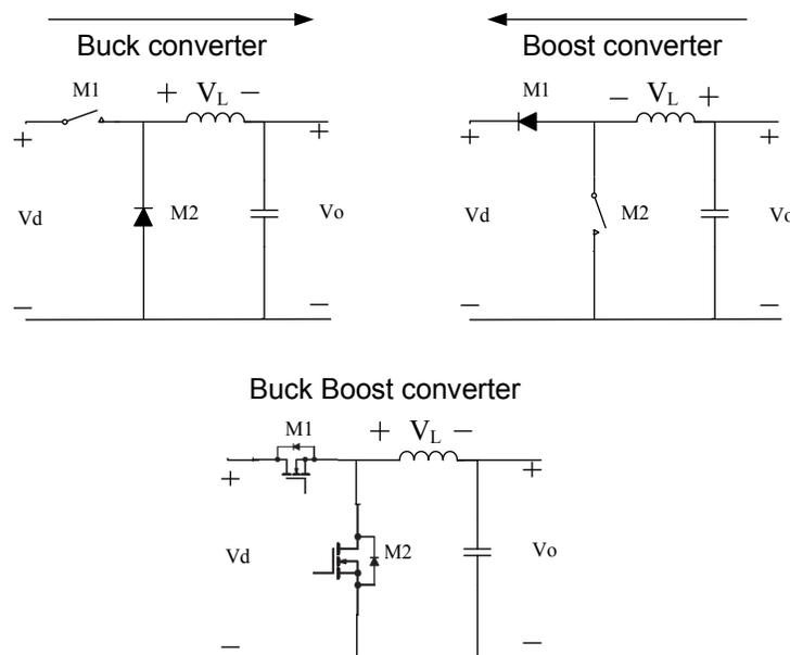
Fig.3. 1 bidirectional Buck-Boost , Buck and Boost converter
