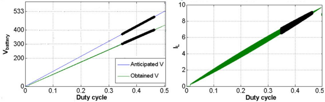
Fig.8. 2 Open loop performance of buck DC-DC converter. Black area indicates the operation area in which the battery voltage may vary (from low SOP to full charge) The width of  $I_L$  represents the expected ripple at corresponding duty cycle
