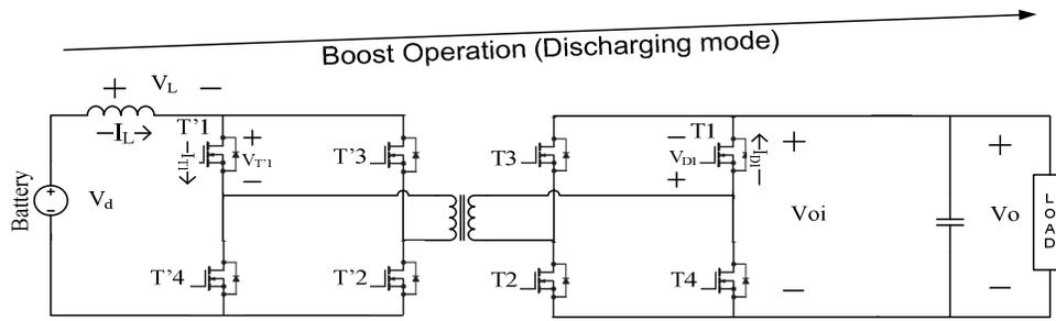
Fig.7. 1 Full-bridge bidirectional converter, when it operates in boost (discharging) mode
