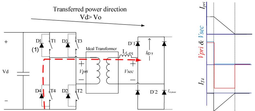
Fig.5. 9 Transformer leakage inductance forces the diodes of primary side to turn-on
