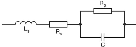
Fig3. 14 Conventional capacitor modelling.
