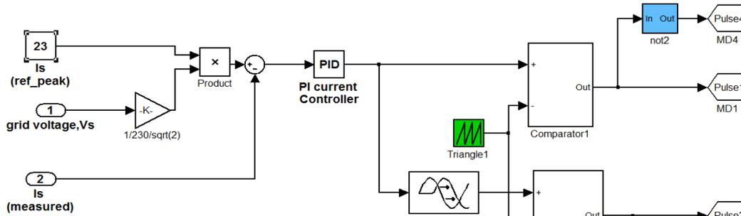
Fig.9. 6 The block diagram of the controller including PWM switching pattern generator of the inverter.
