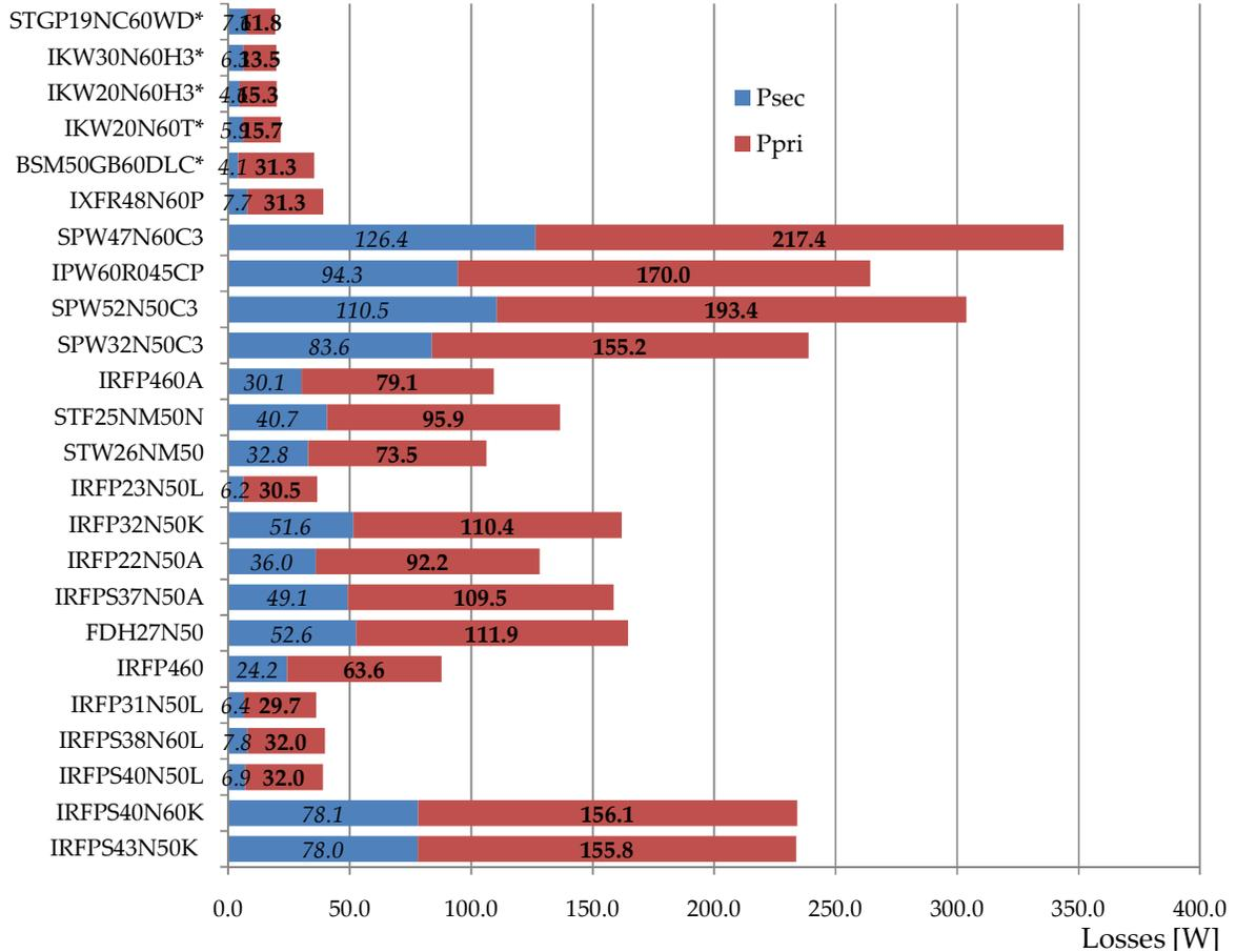
Fig.5. 12 The total switch losses of a single switch in primary and the same switch on secondary side (\*represents IGBT) ( $P_{out}=3600W$ (Switching losses based on  $I_{Gon} = 1.2A$  for all switches (simplified model)
