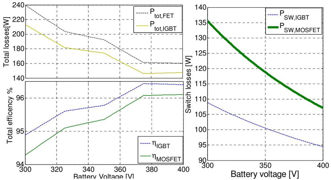
Fig.7. 7 (left-up): DC-DC full bridge boost converter losses. (left -down): Total efficiency of the converter. (right):total switch losses as a function of voltage with two different switches. One IGBT (IKW30N60H3) and one MOSFET(IRFP31N50L)
