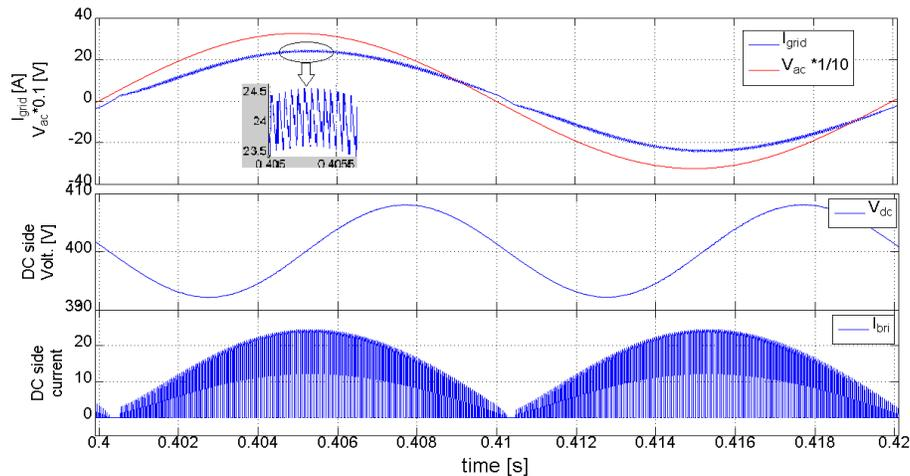
Fig.9. 4 (Up) the input current and grid voltage, (middle) output DC current, (down) Bridge current in DC side, (ref Fig.9. 1.(A))
