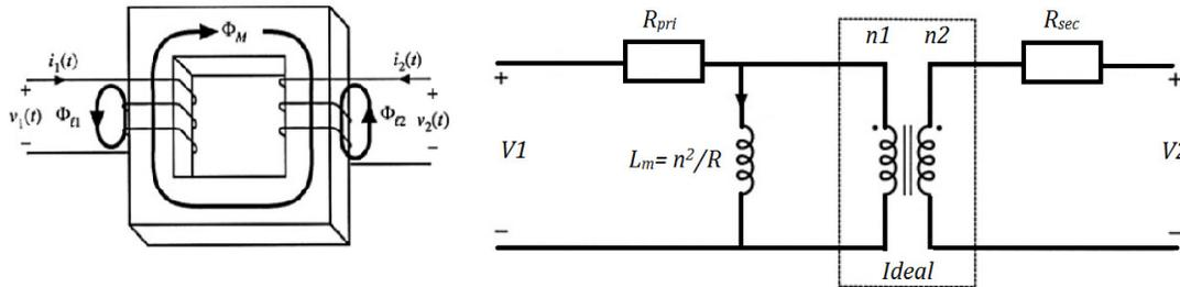
Fig.3. 13 Left: A transformer, windings and core,  $\phi_L$  is the result of leakage inductance . Right: Non ideal model of transformer (including an ideal model)
