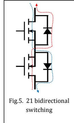
Fig.5. 21 bidirectional switching
