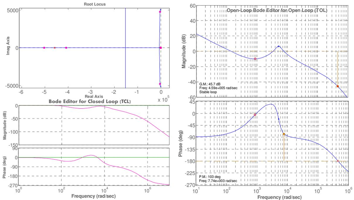
Fig.8. 13 top left: Root locus plot of the system with the compensator, The red squares are the closed-loop poles; x indicates open loop poles. Right) Open loop bode diagram.  $P.M = 103^\circ$ ,  $G.M = 45.7dB$ ,  $w_{cross} = 7.7e3 \text{ rad/sec}$  Down left) closed loop bode diagram of the system.
