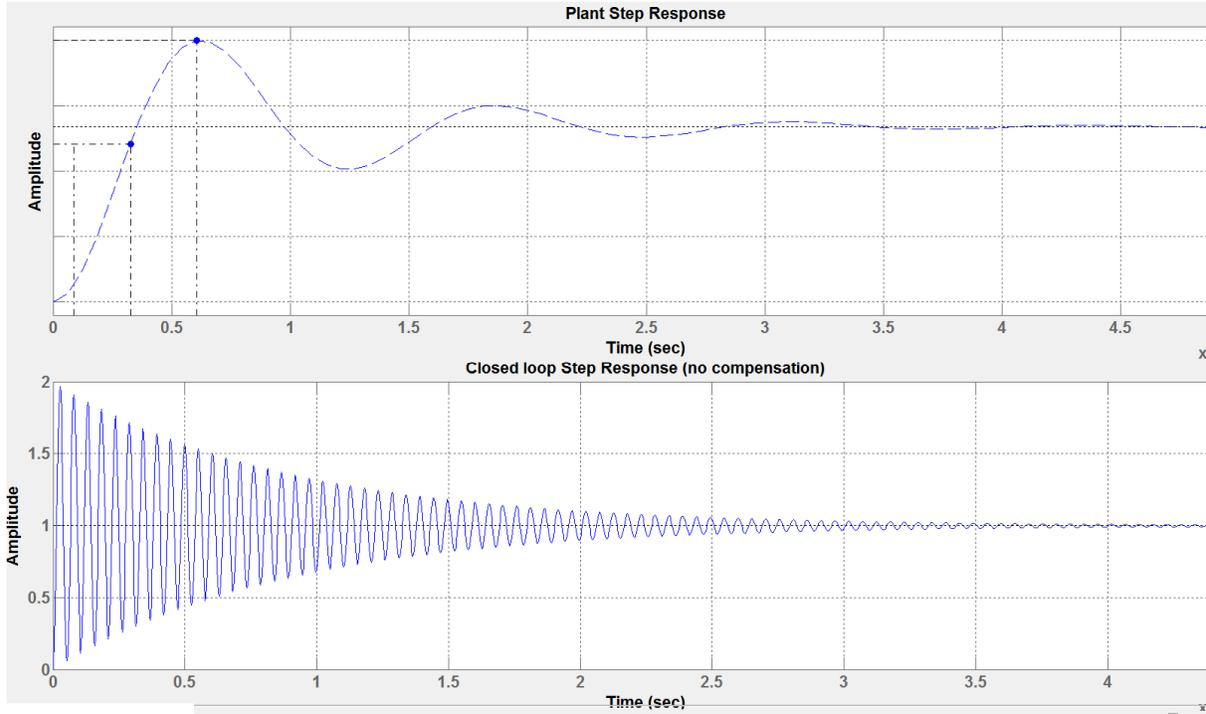
Fig.8. 9 The step response of the transfer function of the full-bridge DC-DC converter,  $T_1(s)$  when  $T_c = T_m(s) = 1$
