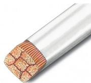
Fig.B. 1 an example of Profile Litz wire with 65-80% copper fill factor which enables winding without bobbin (self bonding enamel / acetate silk) with max available cross section of  $1 \text{ mm}^2$  Courtesy of RUPALIT®<sup>1</sup>
