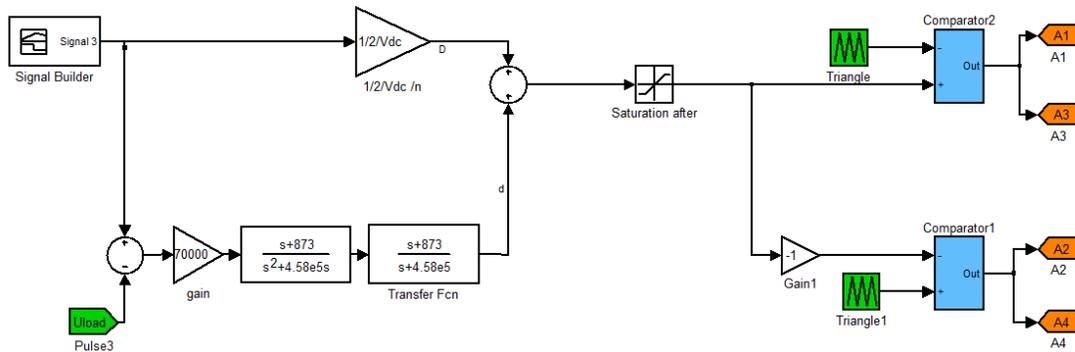
Fig.8. 14 The block diagram and implementation of the type 3 compensator for the DC-DC converter
