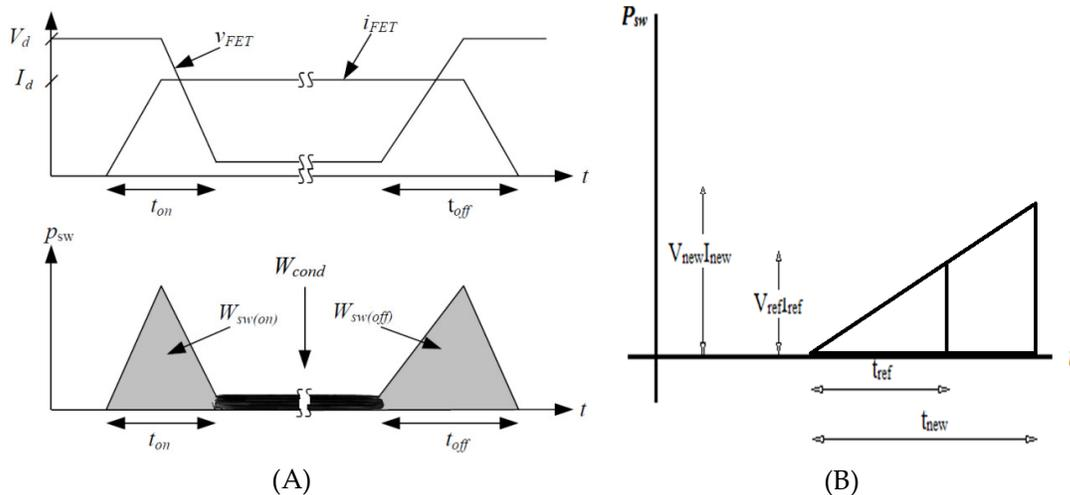
Fig.4. 9. (A) Switch waveforms and energy losses ( $t_{on} = t_{fu} + t_{ri}$ ,  $t_{off} = t_{fi} + t_{ru}$ ), (B) Scaling of current rise time based on reference value,  $t_{ref}$  switching losses
