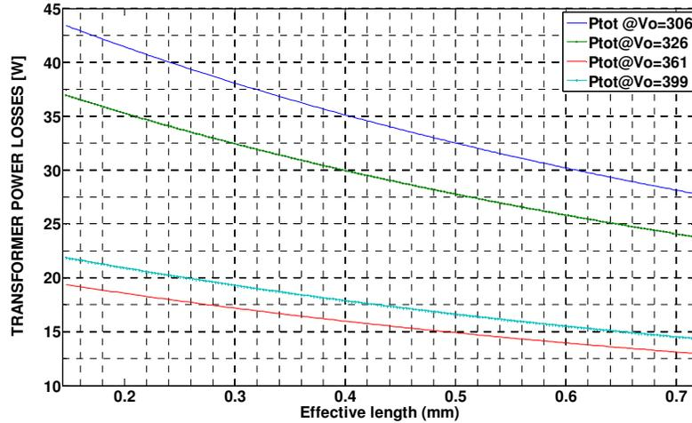
Fig.B. 7 Total transformer losses as a function of core effective length when the core is EC70 ( $N_1 = 30$ ,  $airgap = 1830\mu m$ ,  $\mu r_{3F3} = 2000$ )
