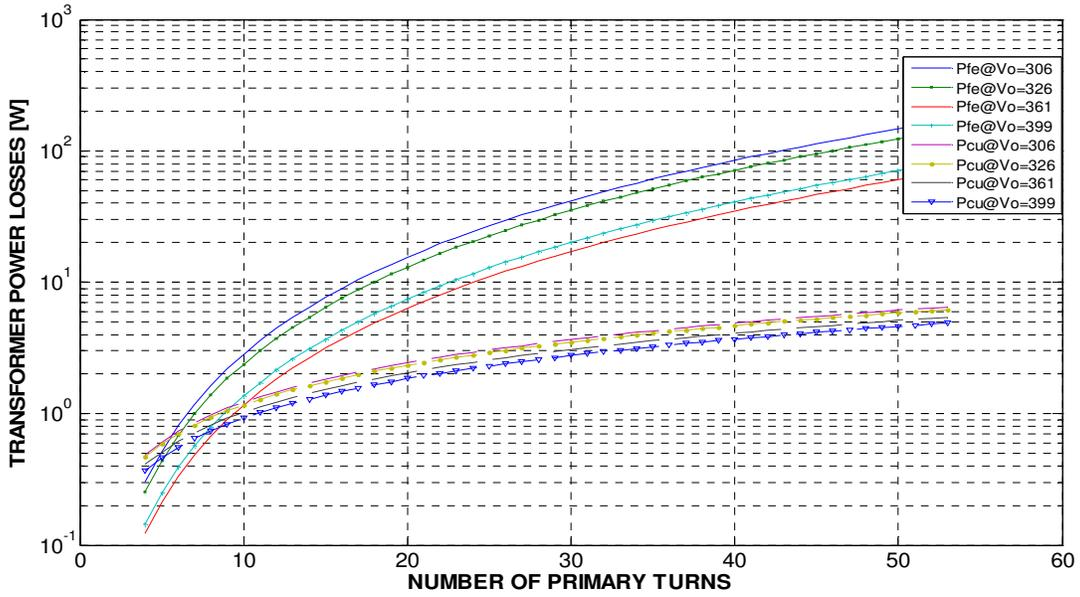
Fig.B. 3 Transformer core and copper losses as a function of number of primary turns when the core is EC70 ( $airgap = 1830 \mu M, \mu r_{3F3} = 2000$ ) (log scale)
