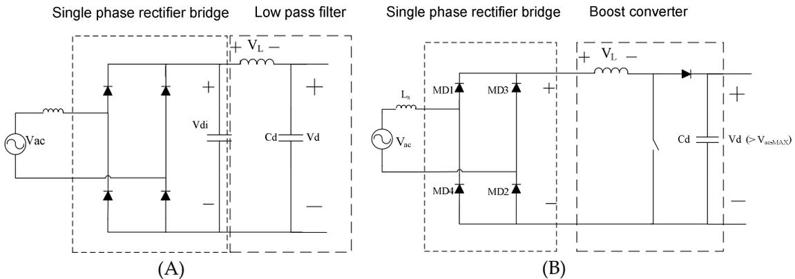
Fig.3. 7(A): Passive PFC circuit (B) unidirectional active PFC. For different topologies and comparisons see: [7]
