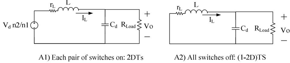
Fig.8. 5 circuit state of (A1) switch-on, and (A2) switch-off
