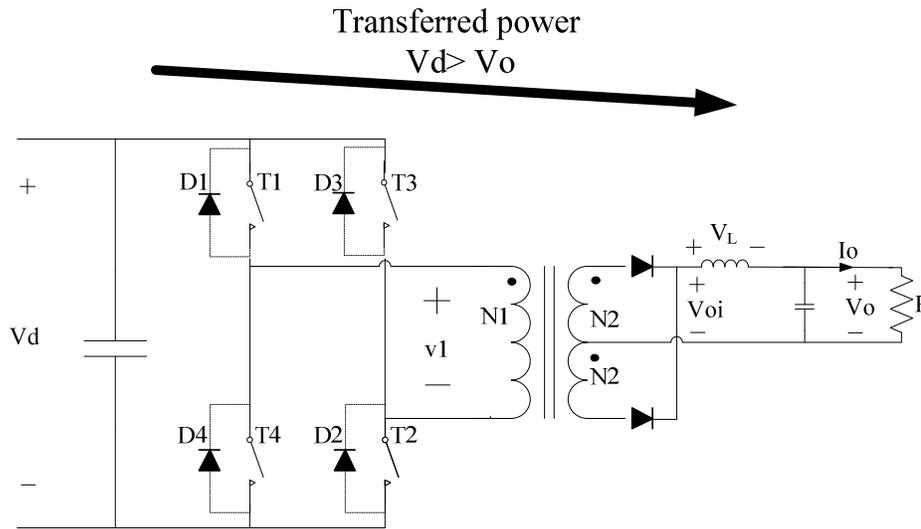
Fig.3. 2 Full-Bridge Voltage Source Converter (FBVSC) with a centertapped transformer
