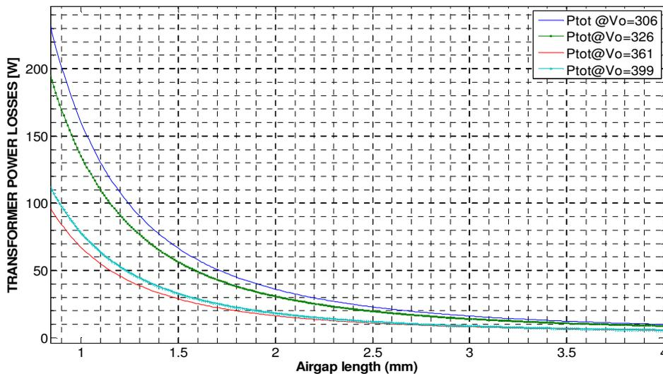
Fig.B. 6 Total transformer losses as a function of airgap length when the core is EC70 ( $N1 = 30, \mu r_{3F3} = 2000$ )
