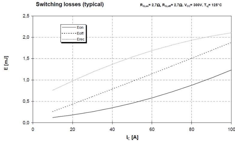
Fig.5. 6 Infineon *BSM50GB60DLCL* switching losses as a function of collector current.  $E_{rec}$ : Recovery losses ([www.infineon.com](http://www.infineon.com))
