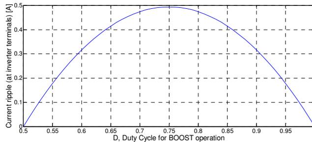
Fig.6. 1 Current ripple in boost operation as a function of duty cycle, when  $L_{ind} = 0.0037 H$
