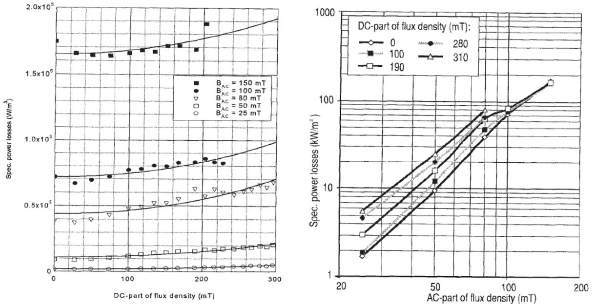
Fig.4. 10 Left: Low loss dependency on the DC part of flux (esp. at low  $B_{ac}$ ) Right: high dependency on  $ac$  part of flux. From Figures 6 and 7 of [20]
