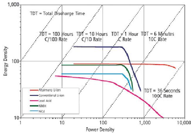
Fig.3. 15 Ragone chart, superior energy density at a certain power density of Li-ion battery
