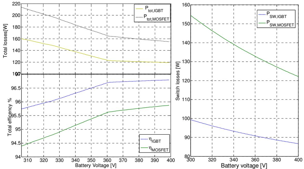
Fig.6. 6 (left-up): DC-DC full bridge buck converter losses. (left -down): Total efficiency of the converter. (right):total switch losses as a function of voltage with two different switches. One IGBT (IKW30N60H3) and one MOSFET (IRFP31N50L)
