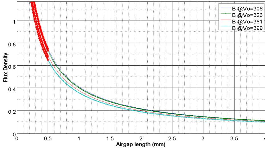
Fig.B. 5 Flux density as a function of airgap length when the core is EC70 ( $N1 = 30, \mu r_{3F3} = 2000$ )
