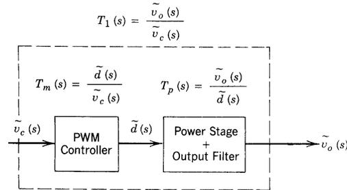
Fig.8. 6 The open loop block diagram of the DC-DC converter
