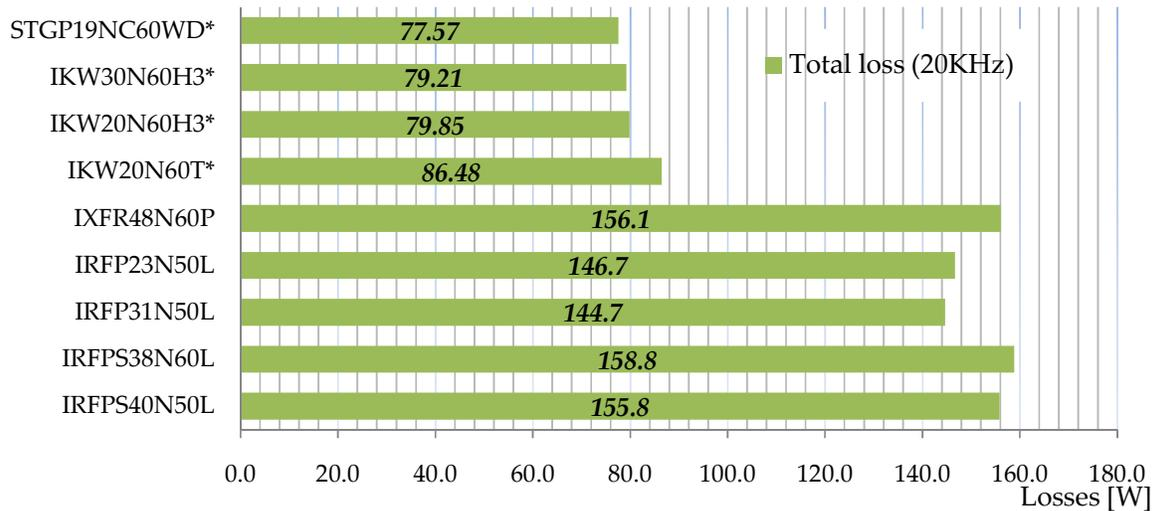
Fig.5. 13 Total switch losses of DC-DC full bridge converter (\* represents IGBTs) ( $P_{out}=3600W$ ) Switching losses based on  $I_{Gon} = 1.2A$  for all MOSFETs
