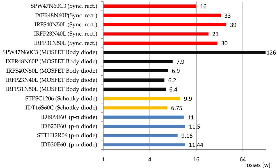
Fig.5. 24 Single switch losses comparison (on secondary side) between SR method, p-n Diodes, Schottky diodes, and MOSFET body diodes ( $V_d=400V$ )
