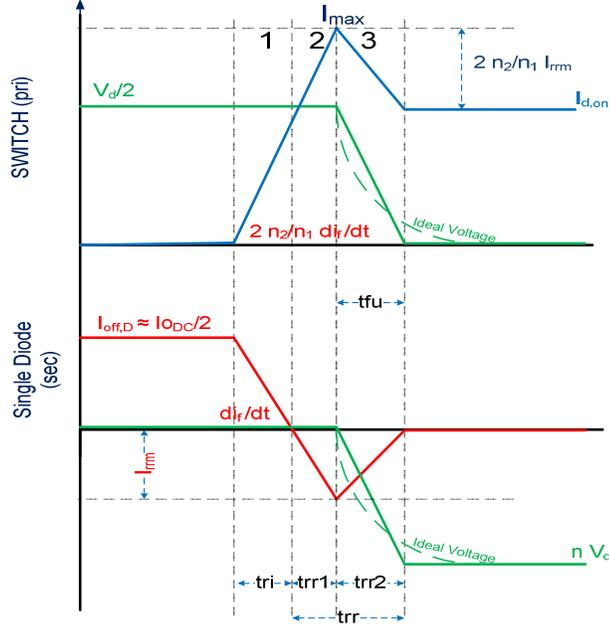
Fig.5. 20 MOSFET Voltage and current during turn-on transient. Down: Diode voltage and current transient during MOSFET turn-on(=Diode turn-off) secondary side of full bridge DC-DC converter
