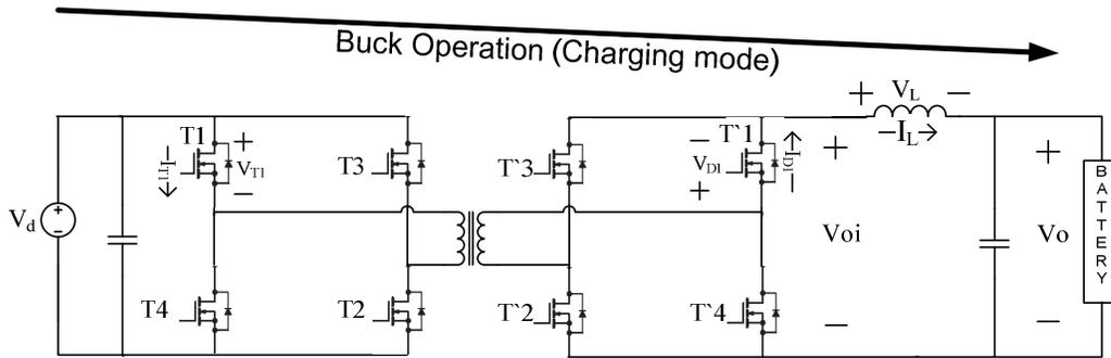
Fig5. 1 Full-bridge bidirectional converter, when it operates in buck (charging) mode
