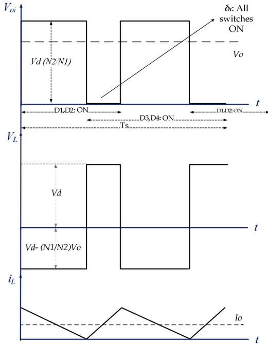
Fig.3. 4 Boost Full-bridge waveforms, Inductor current is shown in boundary conditions (between continuous and discontinuous mode) the parameters are defined in Fig.3. 5
