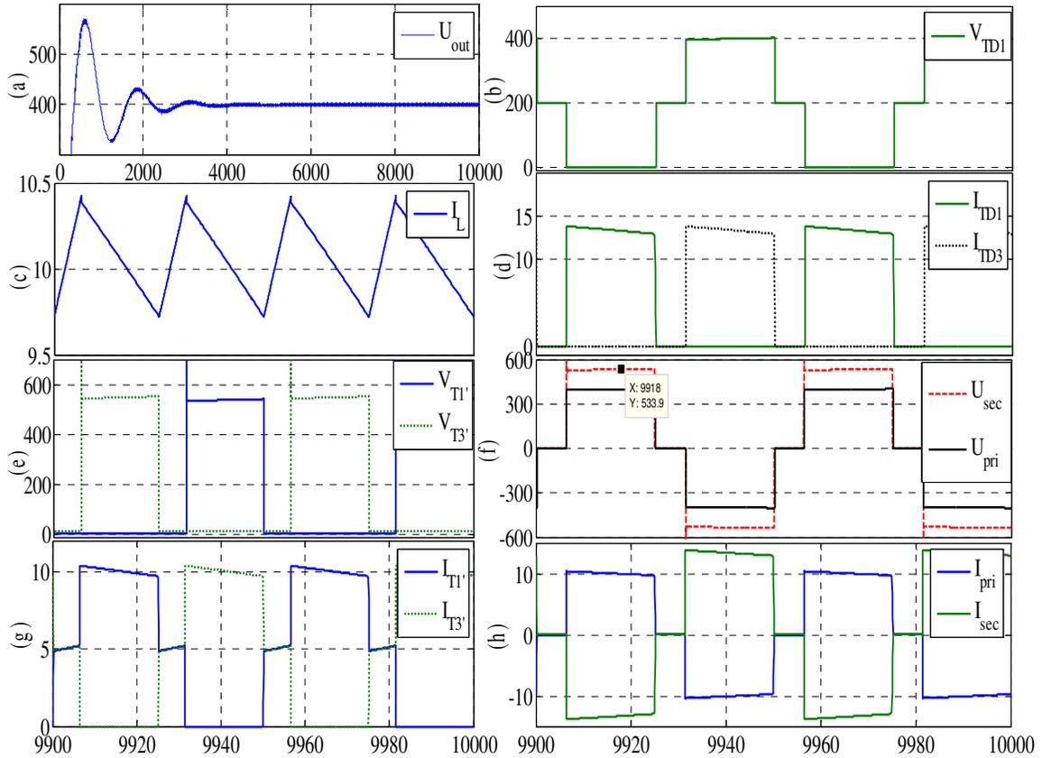
Fig.8. 4 Simulation result of the DC-DC converter and its waveforms, in boost operation mode (dicharging) when the battery voltage and output voltage are 400V. (input power from battery is around 3950 W) (resistive load) In absense of any compensation, large voltage overshoot is abserved.
