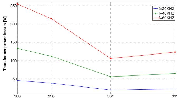
Fig.B. 1 Transformer losses as a function of output voltage (Battery voltage) for different frequencies
