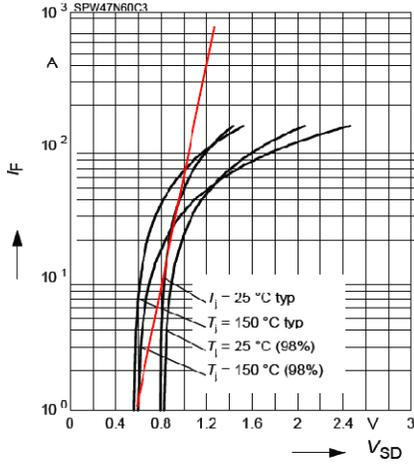
Fig.5. 4 Forward characteristics of body diode,  $T=150 \Rightarrow$  typical.  $U_{d0} = 0.6$ ,  $R_D = \frac{0.4}{16} = 0.025 \text{ ohm}$ . For  $T=25 \Rightarrow$
