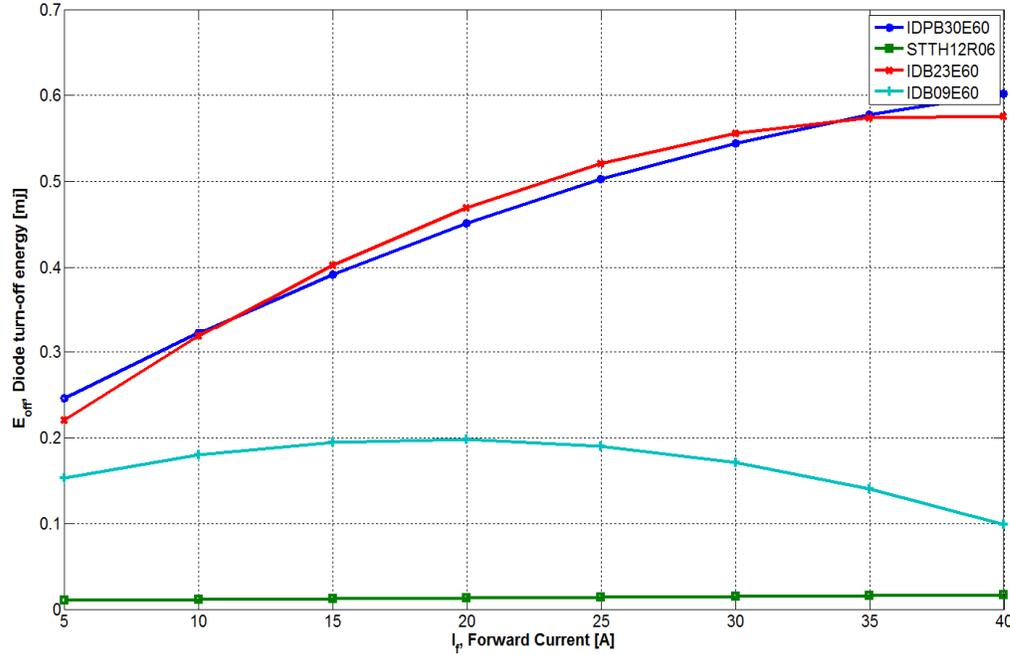
Fig.5. 19 Diode turn-off energy losses of 4 differet p-n diodes as a function of forward current @ dif/dt=200
