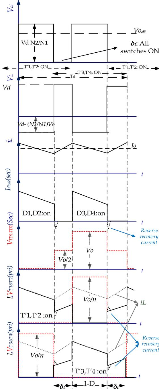
Fig.7. 2 DC-DC fullbridge Boost converter waveforms. The topology can be seen in Fig.7. 1 the principle of operation is explained in chapter 3
