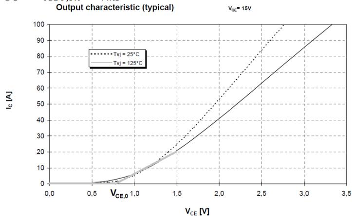
Fig.5. 5 Infineon BSM50GB60DLCL Gray line: linearized output characteristic, here  $V_{CE,0}=0.75 \text{ V}$ ,  $R_{IGBT,ON}=0.75/20=0.375 \text{ ohm}$  (for  $T_{vj}=125$ ) ([www.infineon.com](http://www.infineon.com))
