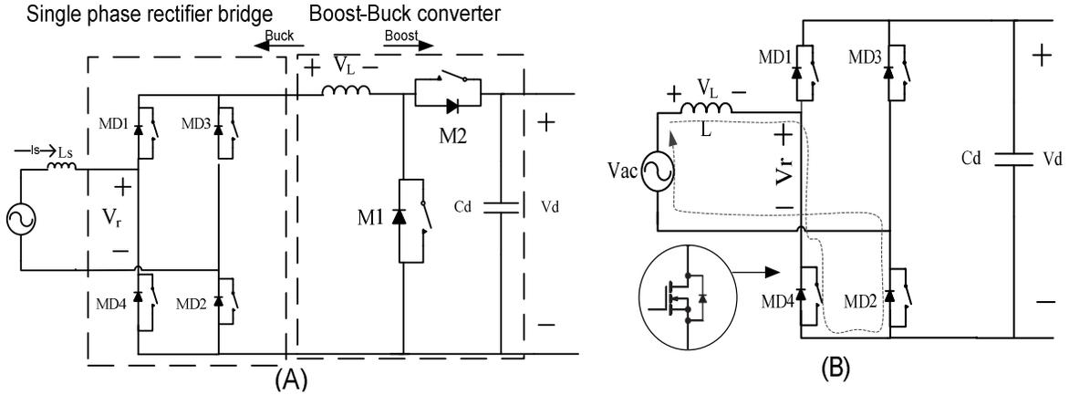
Fig.3. 8 Two different bidirectional APFC circuits. (A) Power Frequency Rectifier (PFR): single phase bridge rectifier +Buck-Boost Converter both will form a Bidirectional ac-DC converter, (B) Switch Mode Rectifier (SMR)
