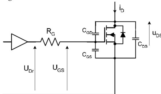
Fig.4. 1 Elements that have the highest influence on switching even of MOSFET. Driving circuit dictates the gate current which charges/discharges the MOSFET capacitances and these capacitances (esp.  $C_{GD}$ ) determine the switching time. The larger the capacitances, the higher switching time thus switching losses.
