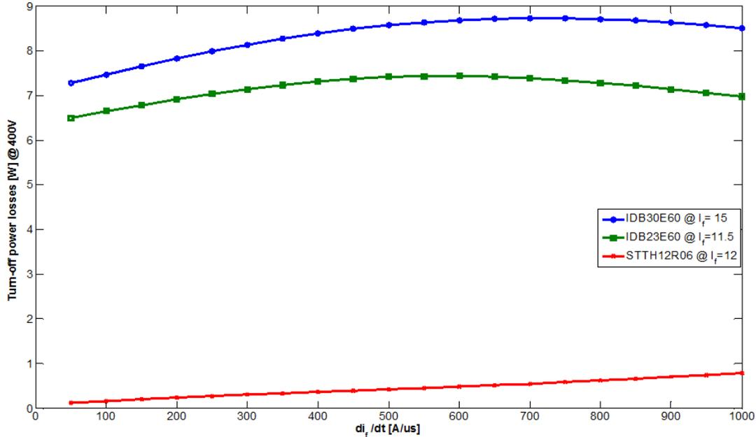
Fig.5. 17 turn-off power losses of 3 different diodes as a function of  $di_f/dt$
