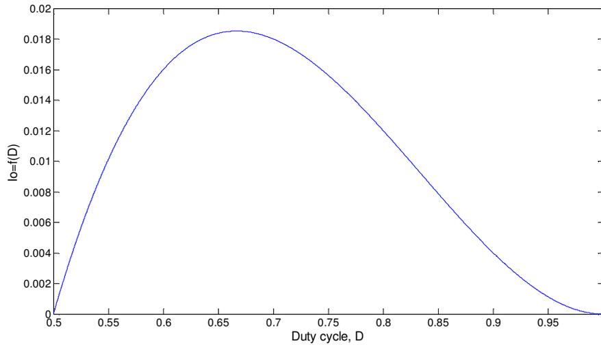
Fig.3. 11 Output current as a function of  $D$  in full bridge boost converter (boundary conditions)
