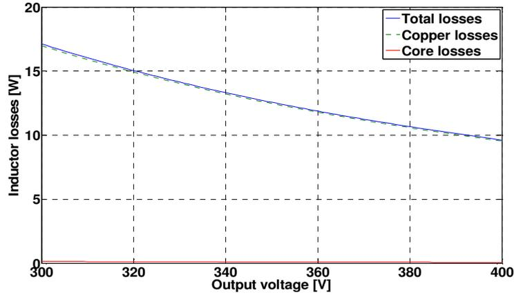
Fig.6. 3 Inductor losses as a function of output voltage (Core: *E713332E250*, Airgap: 5.28mm) at  $P_{out} = 3600W$  and  $f_{sw} = 20kHz$  (core losses are close to zero)
