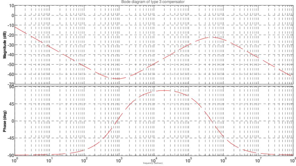
Fig.8. 10 The bode diagram of the type 3 amplifier as a function of frequency (rad/sec), based on the final values found and plugged in (8.36)
