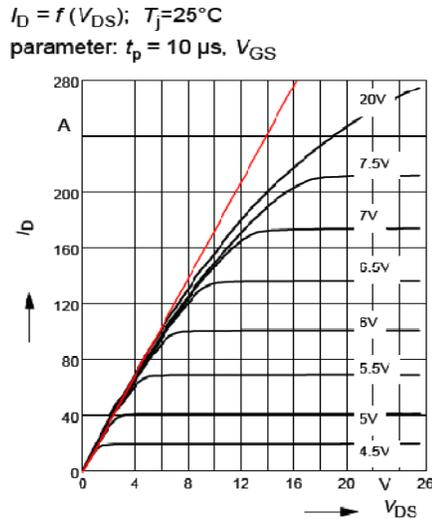
Fig.4. 2 Straight red line: linearized model of MOSFET. We wish the MOSFET operates only in this line in Power electronics applications. the reverse of the red line slope is  $R_{DS(on)}$  ([www.infineon.com](http://www.infineon.com) SPW47N60C3)
