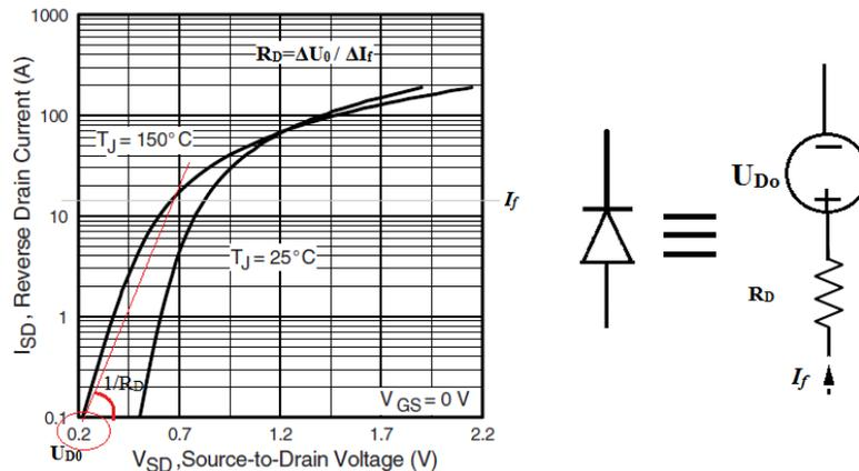
Fig.4. 3 Modelling a diode with DC voltage source ( $u_{D0}$ ) and on-state resistance. Courtesy of Infineon ([www.infineon.com](http://www.infineon.com))
