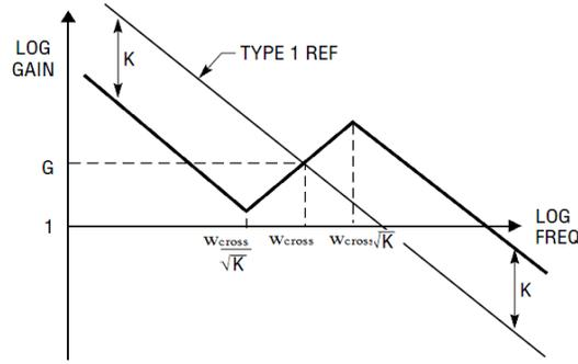
Fig.8. 11 The location of zero-pole pairs, as well as cross over frequency in type 3 amplifier
