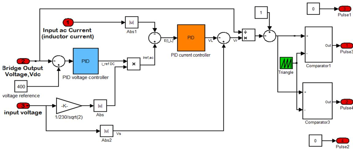
Fig.9. 3 The block diagram of the cascaded controller of the rectifier, the inner loop: PI current controller, outer: PI voltage controller
