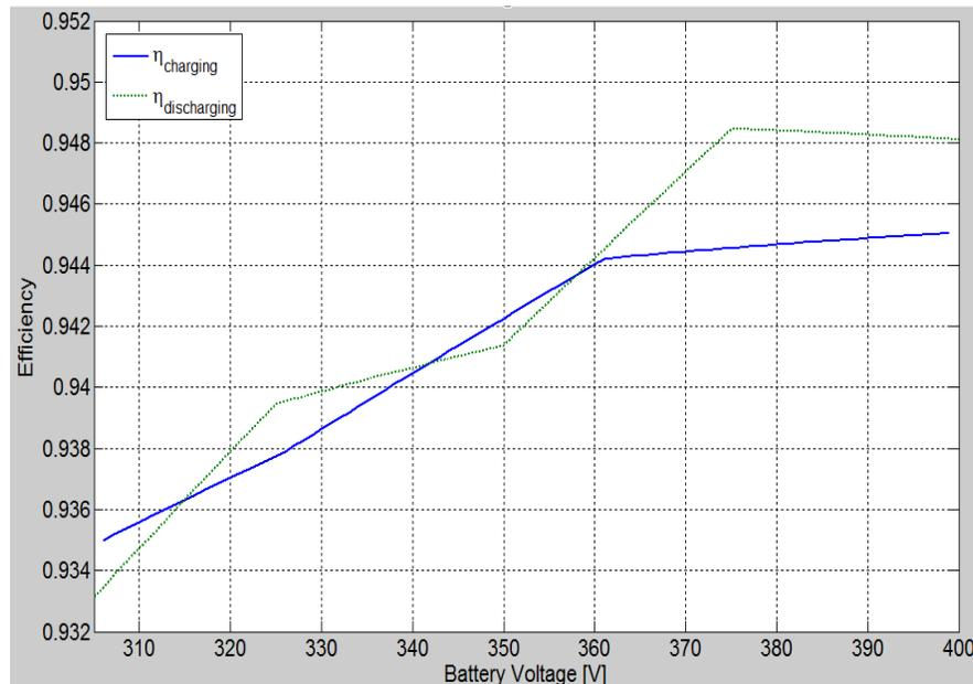
Fig.10. 1 The total efficiency of the onboard charger in both directions, depending on the battery voltage
