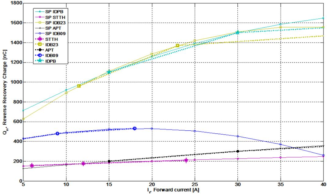
Fig.5. 18 Reverse recovery charge as a function of diode forward current at  $di_F/dt = 200$  A/us (SP: extrapolated lines for  $I_f = 5\sim 10A$ )
