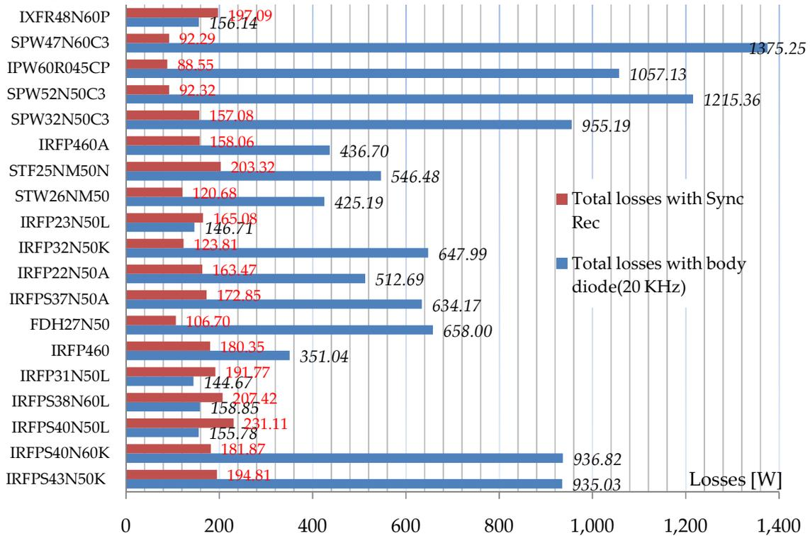
Fig.5. 23 Total switch losses of the DC-DC full-bridge converter with and without Sync. Rec (output power:3.6 KW)
