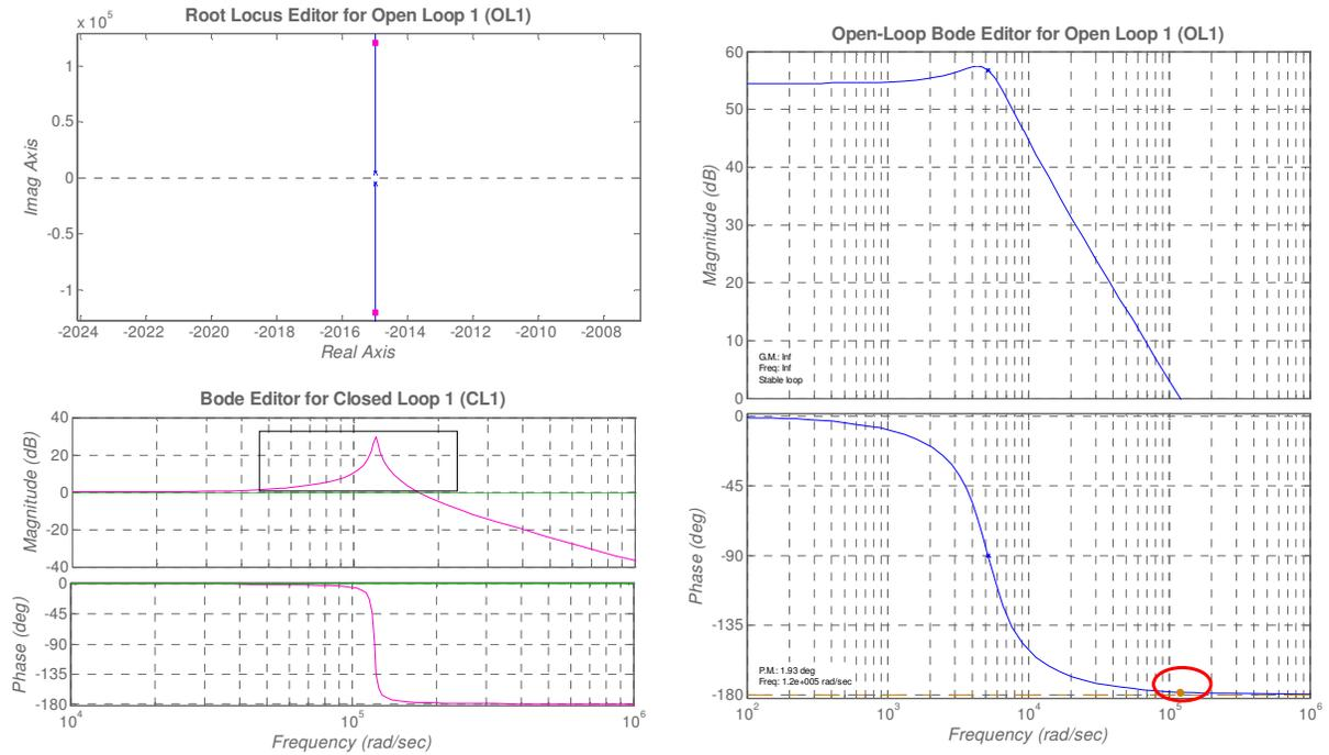
Fig.8. 8 Top left: Root locus plot of the plant when  $K=1$ , The red squares are the closed-loop poles;  $x$  indicates open loop poles. Right) Open loop bode diagram.  $P.M = 1.9^\circ$ ,  $w_{cross} = 1.2e5 \text{ rad/sec}$ . Down left) closed loop bode diagram of the system.
