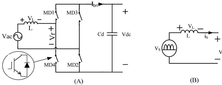
Fig.9. 1 (A) ac -> DC bridge rectifier (B) The equation circuit of the switch frequency bridge rectifier
