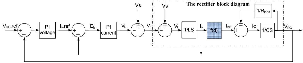
Fig.9. 2 The rectifier block diagram and the linear control system by assuming linear transfer function of rectifier
