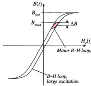
Fig.4. 11 Hysteresis loops: When  $B_{avg}$  is greater than 0, let's say 0.7 p.u, hysteresis loss is the shaded area known as asymmetrical minor loops. Fluctuation of B creates the shaded area (Hysteresis losses)
