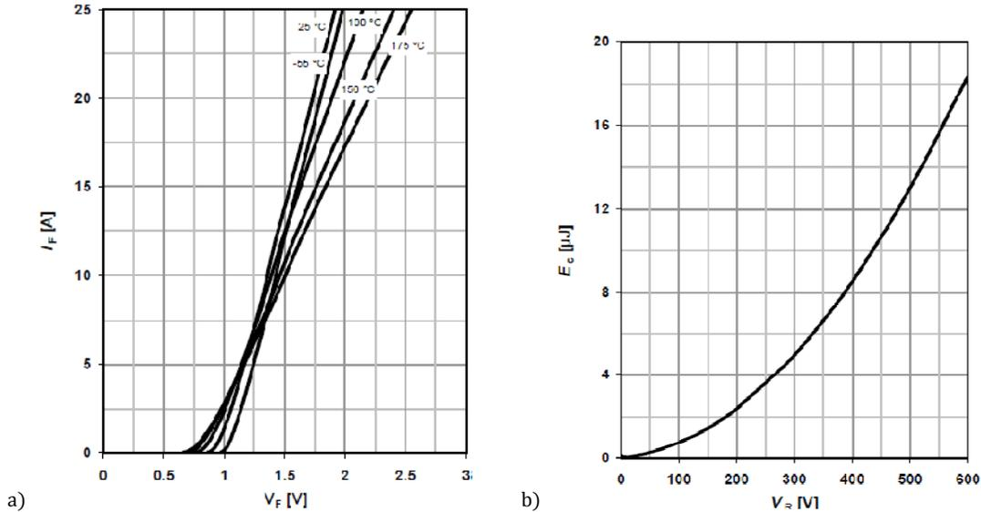
Fig.5. 15 a)  $U_{D0} = 0.9\text{V}, R_D = 0.04 \text{ ohm}$  ( $T=25^\circ\text{C}$ ) b) switching losses in Schottky is only because of junction charge (capacitor). For  $(V_R, E_c) = (400\text{V}, 8\mu\text{J}) \rightarrow P_{sw} = 0.16\text{W}$  (*STPSC1206*, Infineon)
