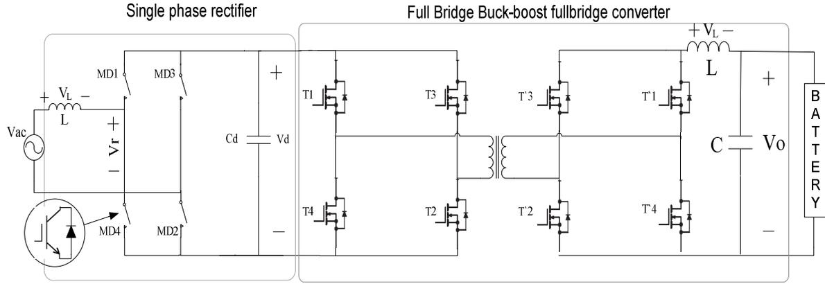
Fig.3. 10 The whole onboard charger topology, including an APFC module and a Bidirectional Full-Bridge DC-DC Converter module
