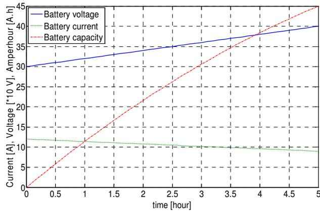
Fig.3. 17 Constant Power Charging method for a  $18kWh$  Li-ion battery
