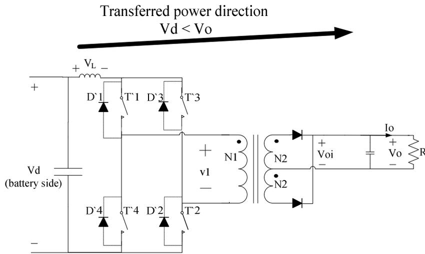
Fig.3. 5 Full-Bridge Boost Current Source Converter topology (FBCSC)
