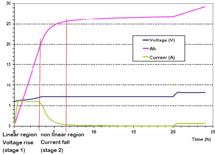
Fig.3. 19 Li-Ion recharging curve of Orvital 6V/24Ah Module. Different Charge stages of a lithium-ion battery can be seen. By courtesy of Dr. Felipe Jimenez , EPISOL project ,Polytechnic University of Madrid (UPM)
