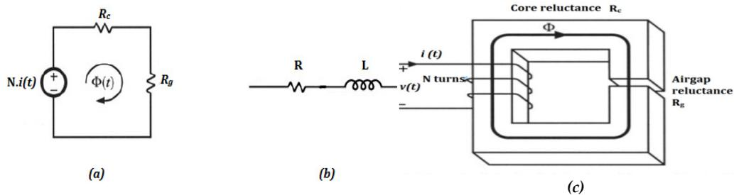
Fig3. 12 Inductance: (a) Magnetic circuit, (b) Electric circuit model of inductor, (c) Simplified structure of filter inductance.
