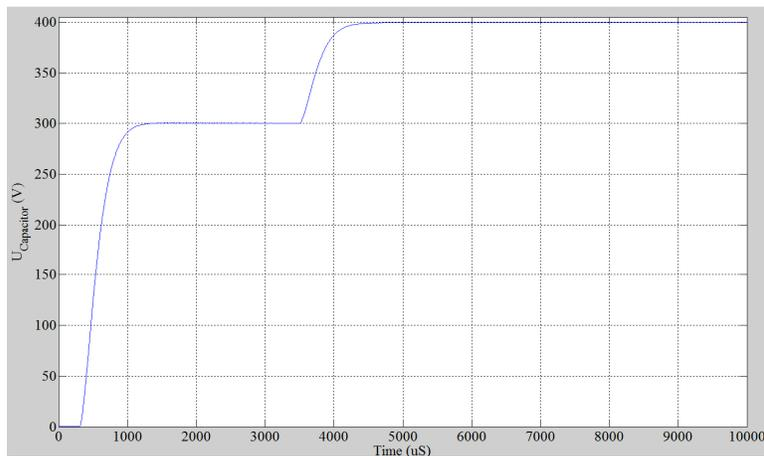
Fig.8. 15 Output voltage Step response of the DC-DC converter, at  $t = 300 \text{ us}$  a step of 300 V is applied. At  $t = 3700 \text{ us}$ , another step, with amplitude of 100V is applied. No overshoot can be observed.
