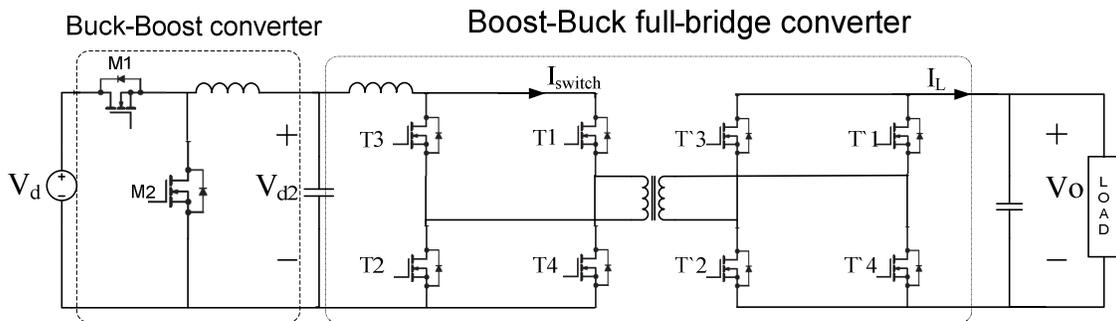
Fig.2. 2 a Bidirectional DC-DC converter topology with galvanic isolation.  $V_o$  can be higher or lower than  $V_d$
