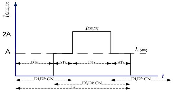
Fig.5. 3 The Simplified current profile of D3 & D4 on the Secondary side, a period can be expressed by  $2\Delta + 2D = 1$
