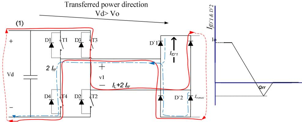
Fig.5. 8 The direction of reverse recovery current in primary side (blue dashed line) As the inductor current cannot change suddenly, the reverse recovery current dose not pass through the inductor in secondary side (see section 7.4.1)
