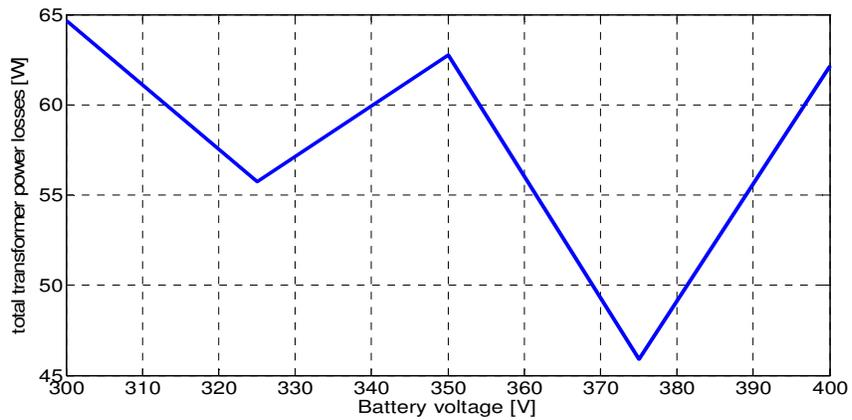
Fig.7. 5 Transformer total losses as a function of battery voltage (Core: *EC70*, Airgap: 1.83mm) at  $P_{bat} = 4000W$  and  $f_{sw} = 20kHz$
