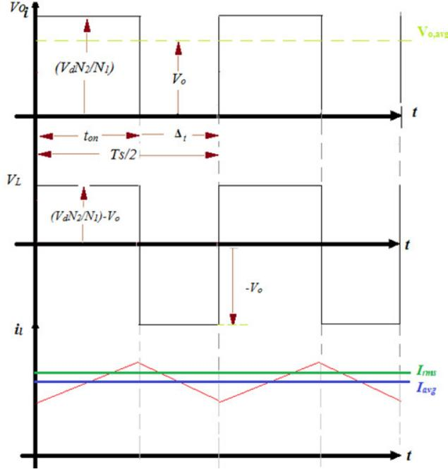
Fig.3. 3 Buck Full-Bridge wave forms
