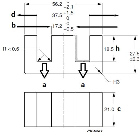
Fig.B. 2 Gray area, Bobbin area. These values are for half core. For full core h should be doubled. From the E55/28/21 datasheet
