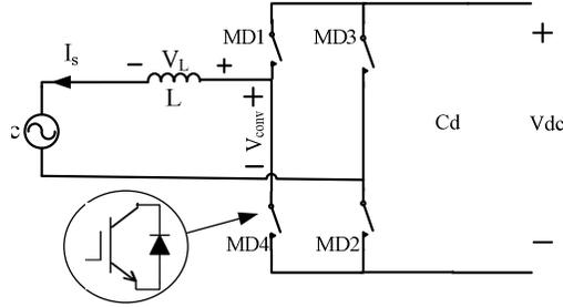
Fig.9. 5 the topology of the inverter in discharging more, when the power is transmitted from DC side to the grid
