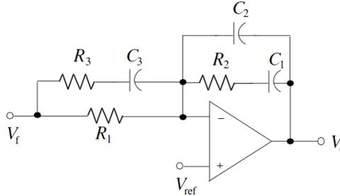
Fig.8. 12 Electrical implementation of type 3 amplifier
