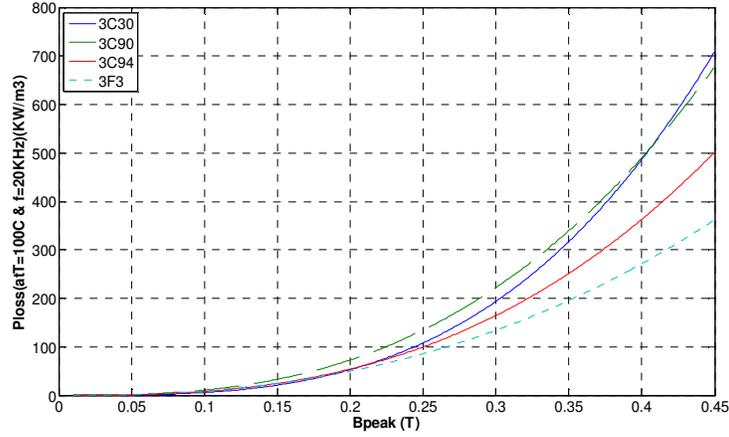
Fig.4. 13 core losses as a function of flux density
