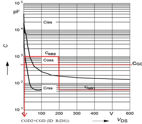
Fig.4. 7 Drain-gate Capacitance as a function of  $V_{DS}$ ; two point demonstration and final selected value:  $C_{GD}$
