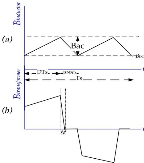
Fig.4. 12 Typical Flux density waveform of (a) inductor (b) transformer. In the inductor, the DC component of flux is neglected. For transformer,  $dB/dt$  in switching transients is so high. The effect of leakage inductance can be seen. (core permeability within its limits is considered as constant) The simulation results also complies with [10]
