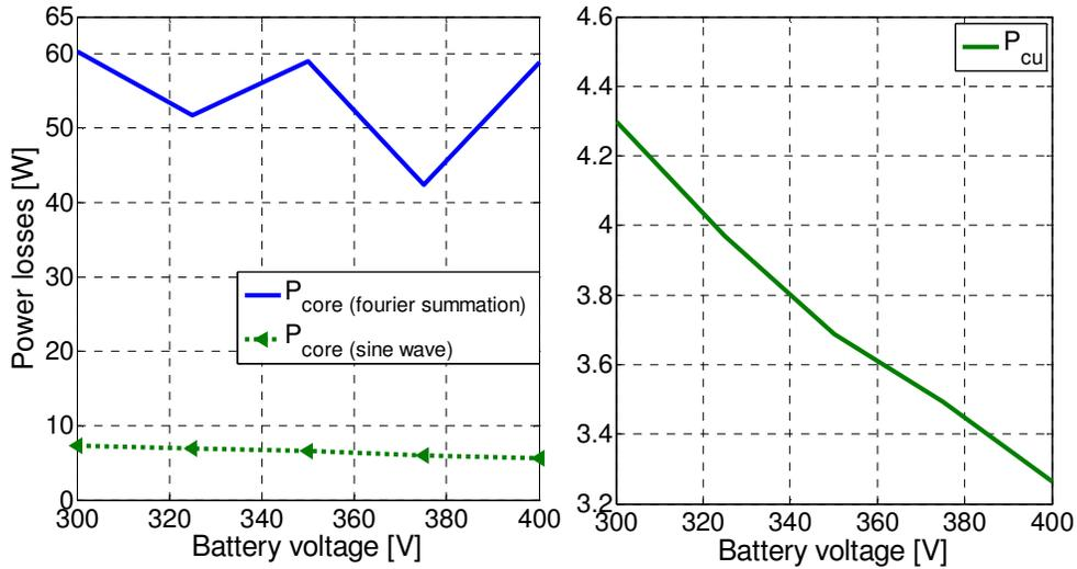
Fig.7. 4 Transformer losses as a function of battery voltage (Core: *EC70*, Airgap: 1.83mm) at  $P_{bat} = 4000W$  and  $f_{sw} = 20kHz$  (Left) core losses with two different method (Right) copper losses
