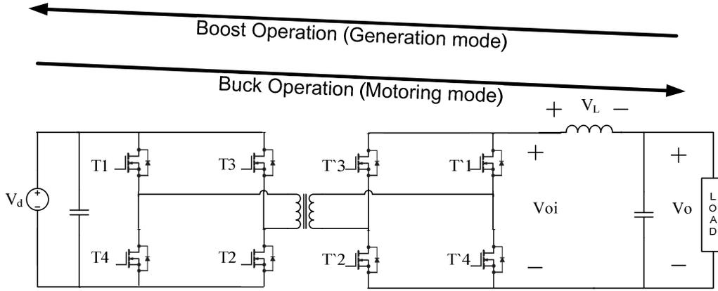
Fig.3. 6 Bidirectional Double-Leg Full-Bridge DC-DC Converter topology
